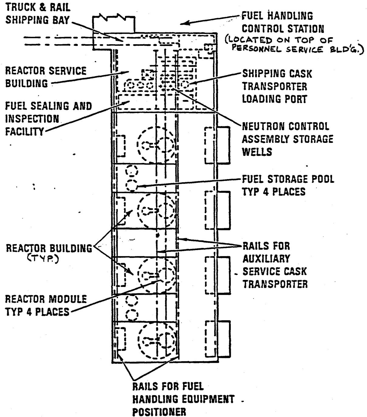
Figure 2-2 SITE FUEL HANDLING – GENERAL ARRANGEMENT
