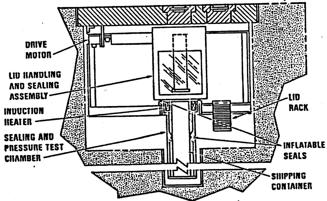
Figure 2-6 FUEL SEALING EQUIPMENT
