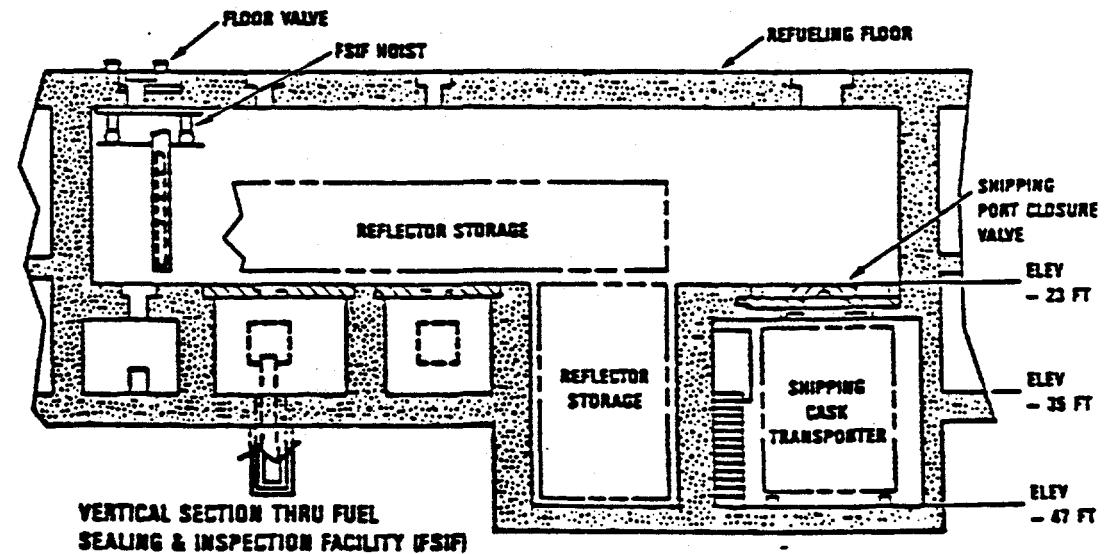
Figure 2-3 SITE FUEL HANDLING – REACTOR SERVICE BUILDING
