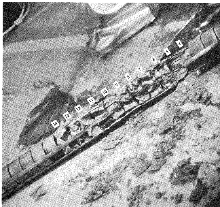
Fig. 76 - Over-all damage to fuel cartridge 1060, cell 273
