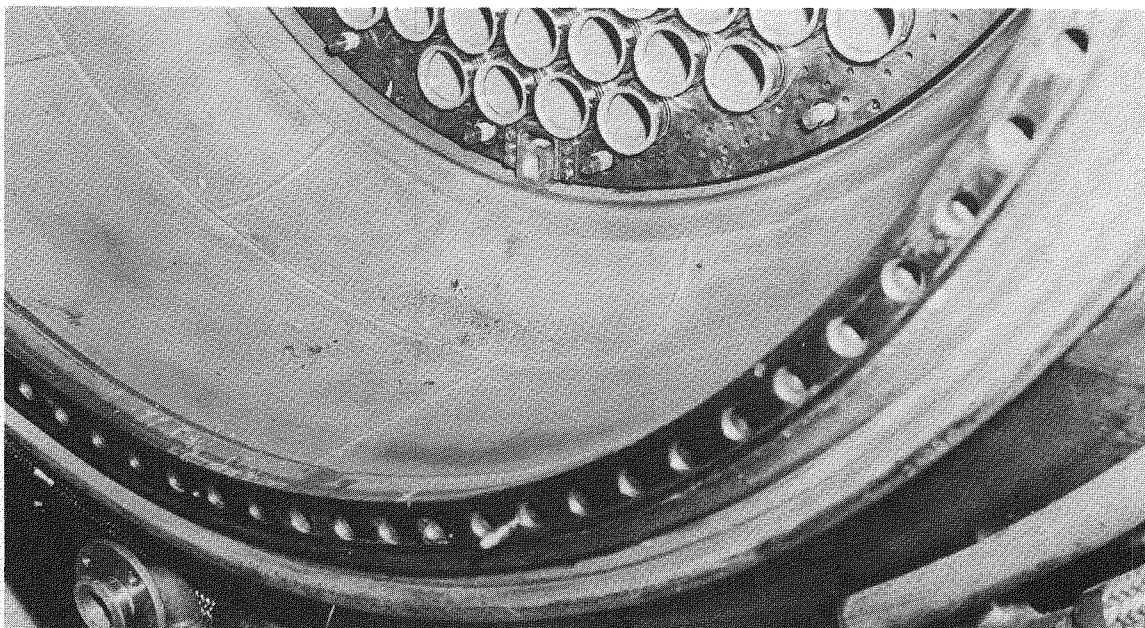
Fig. 109 – Deposits at bottom of primary shield
