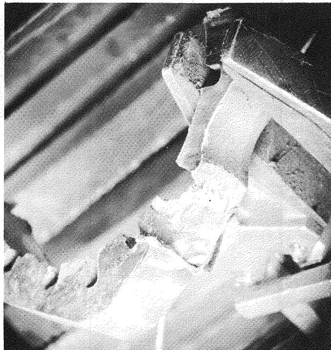
Fig. 101 – Cross section of moderator showing melting and burning damage
