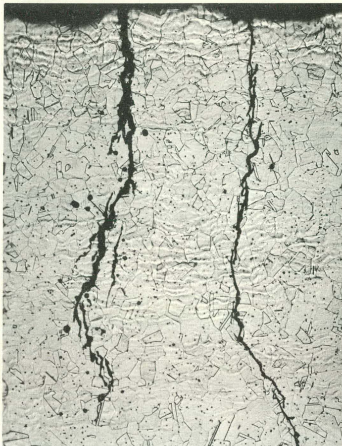
Figure 19. Section Through Hot-Leg of the CL-4 Desuperheater Coil Showing Transgranu- lar Cracks, 60% Nitric Acid Electrolytic Etch 250X
