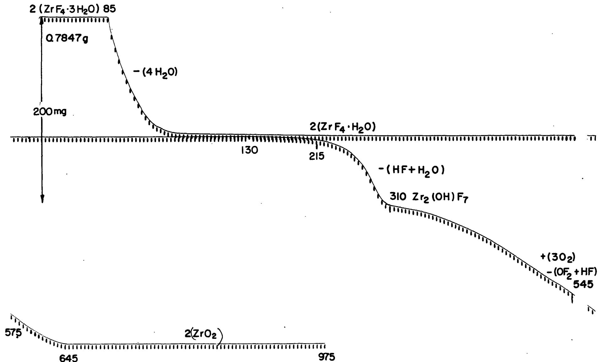
Fig. 2 - Photograph - Thermolysis of Zirconium Tetrafluoride Trihydrate in Air.
