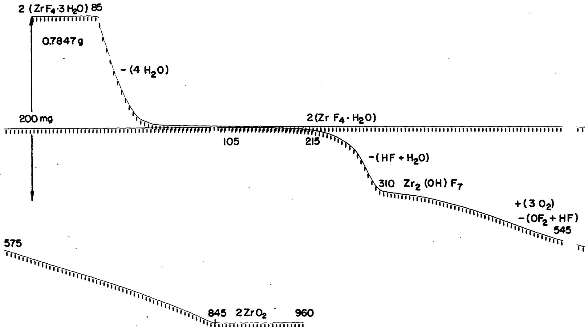
Fig. 1. Photograph - Thermolysis of Zirconium Tetrafluoride Trihydrate in Air.
