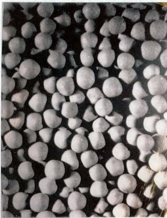
Fig. 3a. Fully coated fuel beads. Oblique incident light at X15.
