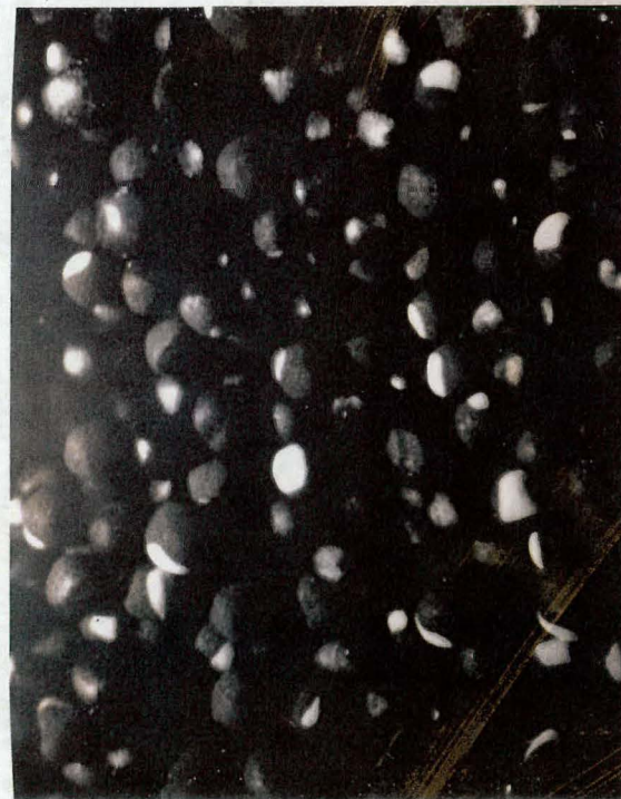
Fig. 4b. Beads after 4 hrs. in \text{Cl}_2 at 950C. Both dull and shiny beads can be seen as well as white spots. Oblique incident light X20.
