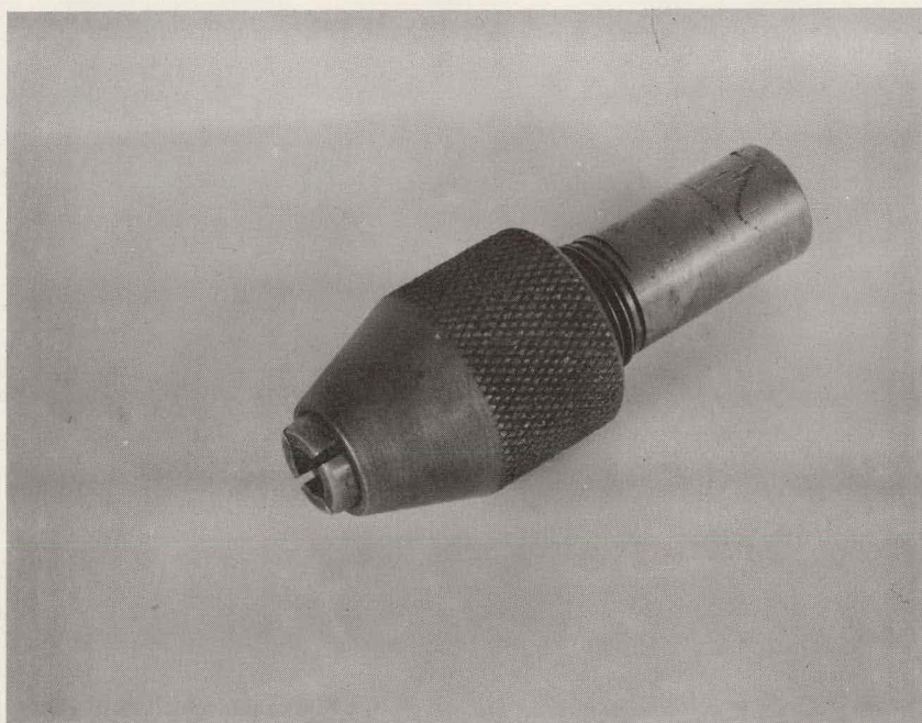
Fig. 18... Collet Type Chill Used to Improve Heat Balance
