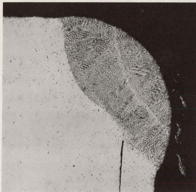
Fig. 21... Shoulder Type Cap Welded without Proper Chill
