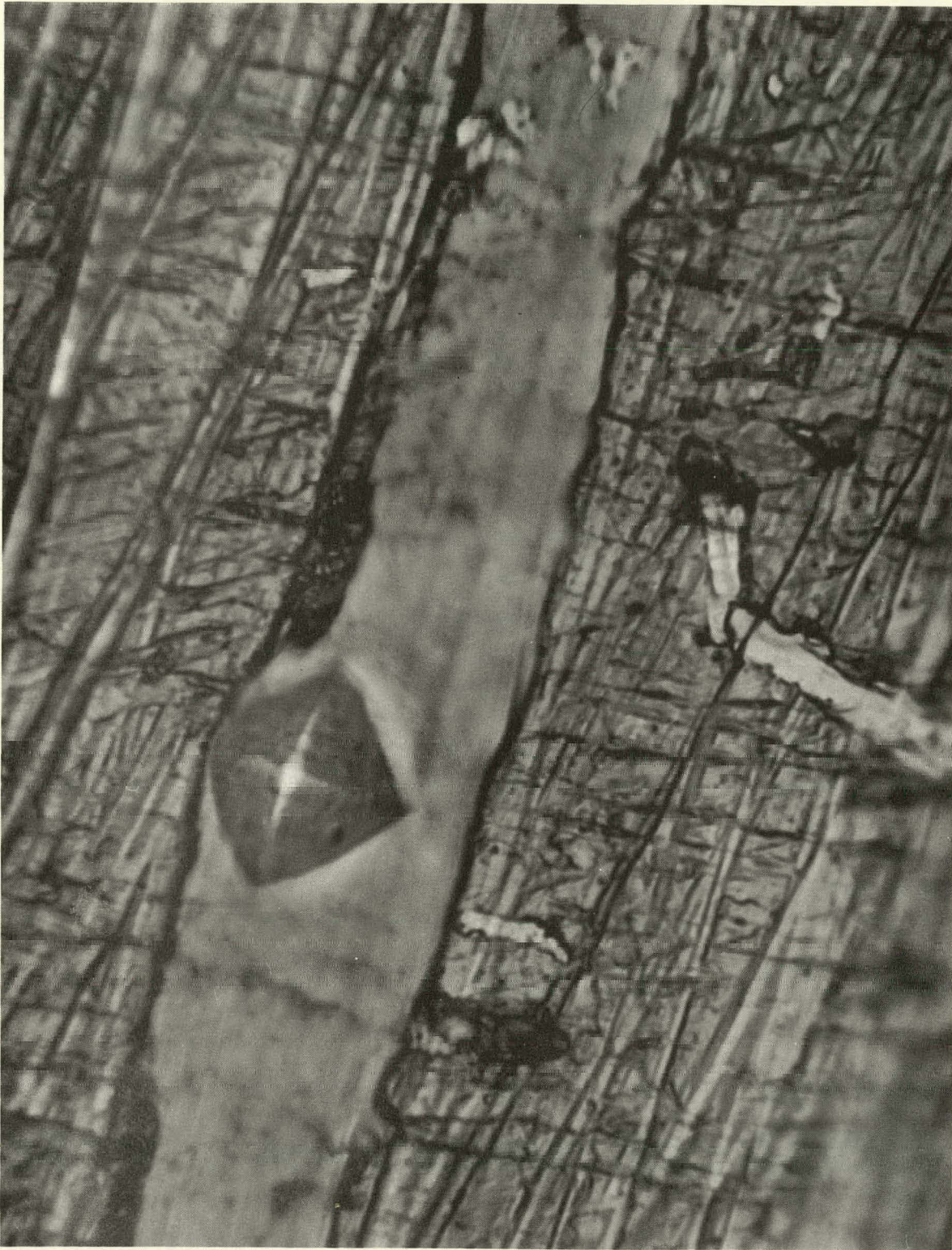
Fig. 1--Light micrograph of rolled tantalum single crystal showing area almost free of slip markings
