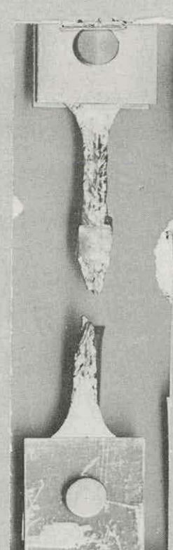
Diffusion Bonded Specimen After Rupture Test
