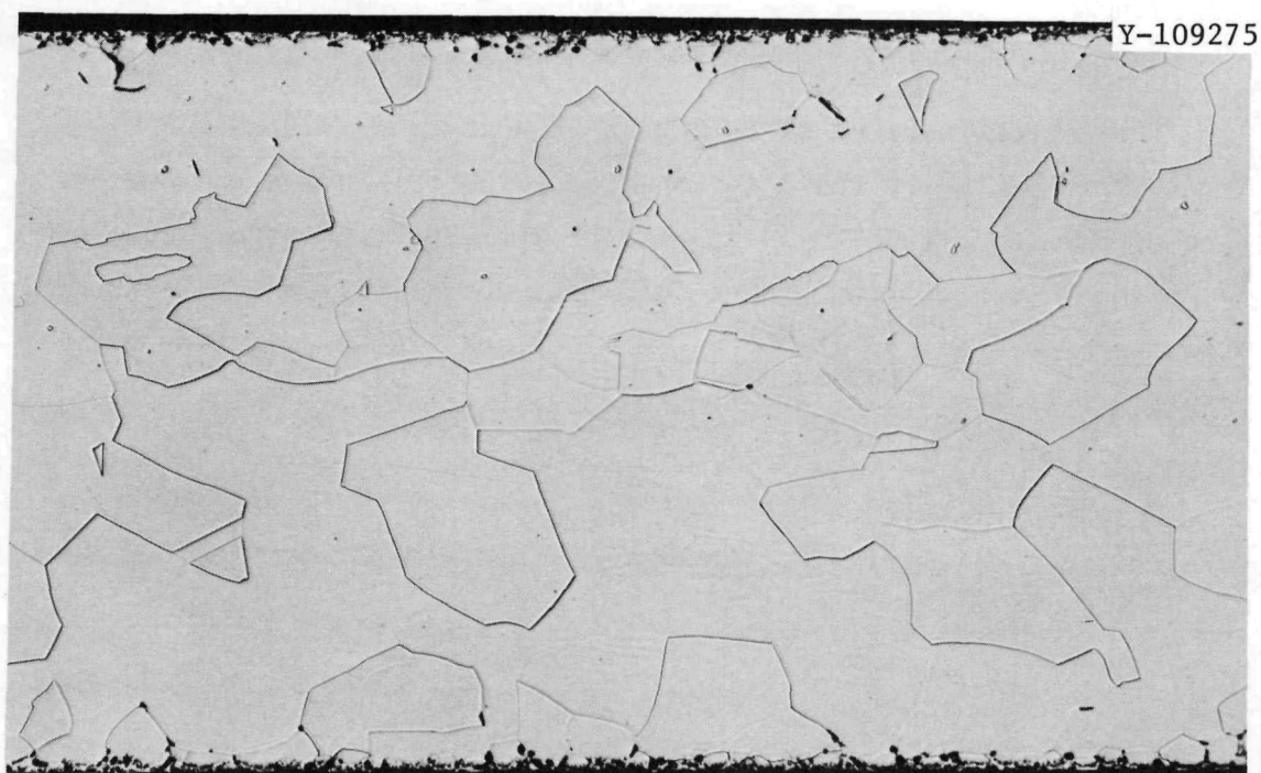
Fig. 17. Alloy Pt-30% Rh-10% W Oxidized 159 hr at 1200°C. Electrolytically etched at 6 V ac for 1.5 min in 80 parts H 2 O:20 parts HCl in saturated HCl. 150×.
