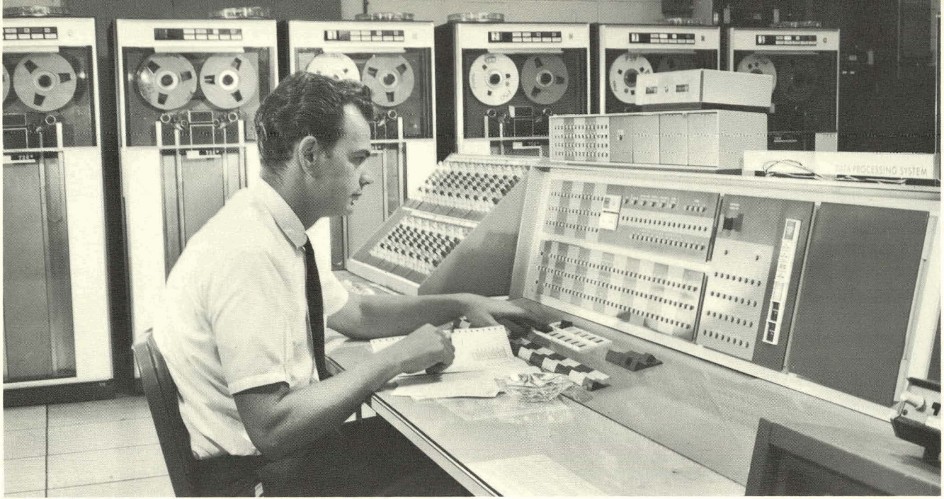
Figure 4. Part of the Laboratory's IBM 7094 data-processing system, operated by the Applied Mathematics Department since 1962. The operator is seated at the console control unit. The lights on the vertical panels and the switches or keys near the operator's left hand provide some of the facilities for man-machine interaction. In the background is a bank of magnetic tape drives; a tape-switching device at the left of the operator enables him to direct the use of all tape drives from one central position. In the lower right-hand corner stands the 21-in. cathode-ray-tube (CRT) visual display. The computer has direct control over this and the associated CRT camera recorder which record and display graphical output generated by the computer program.
