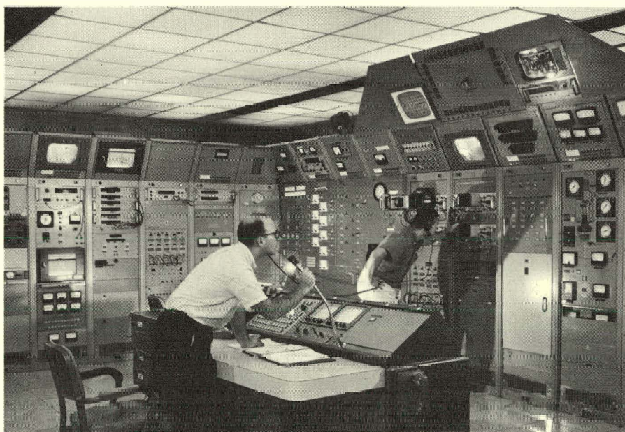
Figure 8. View of the control room of the 80-in. liquid hydrogen bubble chamber, showing some of the many instruments and controls required to monitor and precisely regulate the operation of the large, complex components and systems constituting the bubble chamber.
