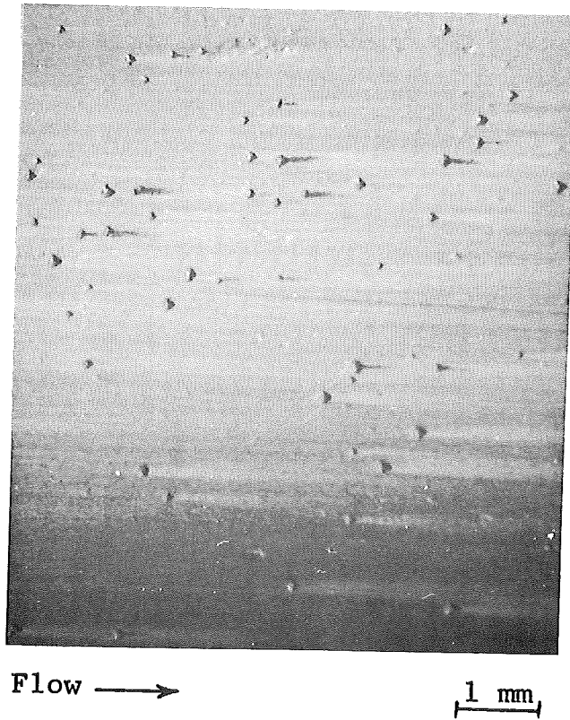
Flow \longrightarrow 1 mm FIGURE 5. Deposit on Section 1-2B after 476 hr operation at T_s = 505^\circ\text{C} plus 149 hr operation at T_s = 536^\circ\text{C} and coolant velocity of 1.5 m/sec.
