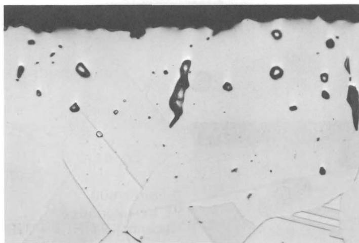
Haynes Alloy 25 71 hr exposure Etchant: \text{HCl} - \text{H}_2\text{O}_2 4L1826
