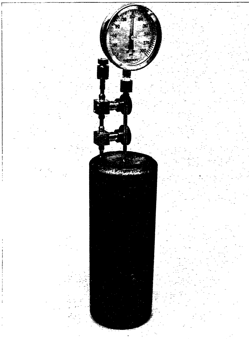
Figure 5-2. Seal-welded test container, fully charged, ready for placement in oven.
