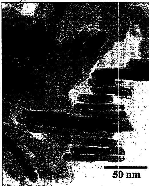
Figure 7: TEM micrograph of BHF particles produced from 0.05 M \text{Fe}^{+3} (from nano-g sol) and 0.05 M \text{Ba}(\text{OH})_2 suspension placed in a 250°C furnace for 48 hours.
