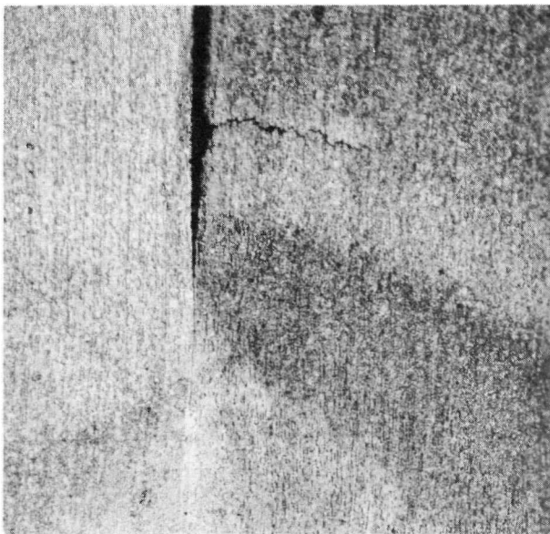
c. Crack in Heat-affected Zone of Weld Bead (unacceptable, not detectable by nondestructive testing)
