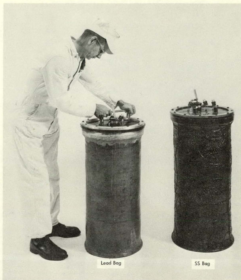
Figure 53. LEAD AND STAINLESS STEEL TEST BAGS AFTER HOT Pressing.
