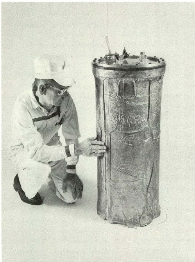
Figure 39. COPPER HOT-PRESSING BAG ASSEMBLY AFTER USAGE.
