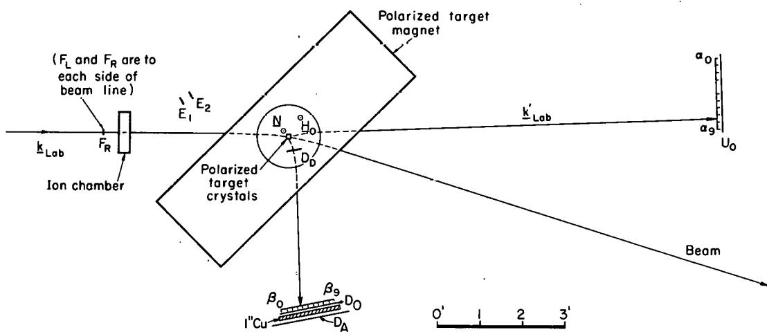
Fig. 8. Arrangement of the scintillation counters. The counter dimensions were:
