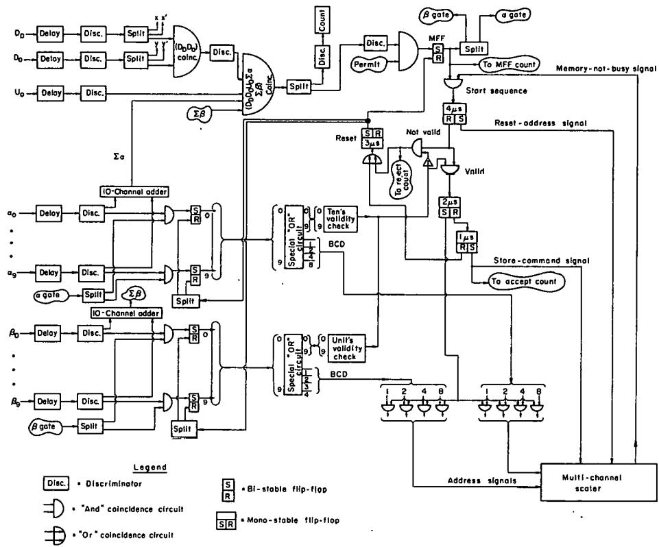
Fig. 9(a). Schematic of electronics used to process and store data.
