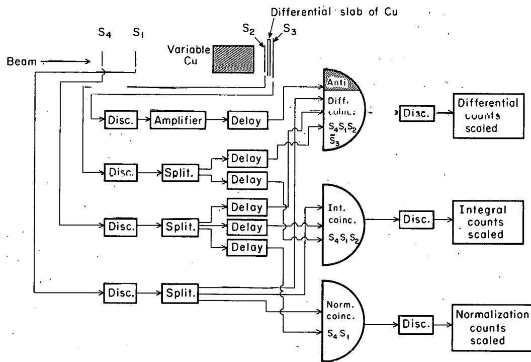
Fig. 2. Range counter-telescope with associated electronics. Counter dimensions were:
