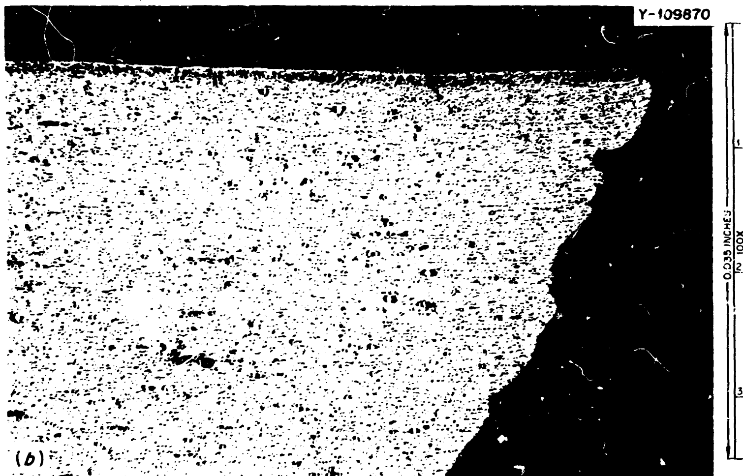
Fig. 7. Microstructure of INOR-8 Sample Held Above 500°C for 3306 hr During the "Zero-power" Run of the MSRE. (Fuel was in system 1090 hr.) (a) As polished. (b) Etched with glyceria regia. The material is cold worked, and the grains are not delineated by etching.
