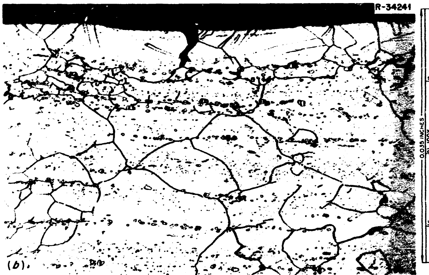
Fig. 11. Photomicrographs of Surveillance Specimen A-16 from Heat 5085 Tested at 25°C and at a Strain Rate of 0.05/min. (a) Fracture. (b) Edge of Specimen about 1/4 in. from fracture. Etchant: glyceria regia.
