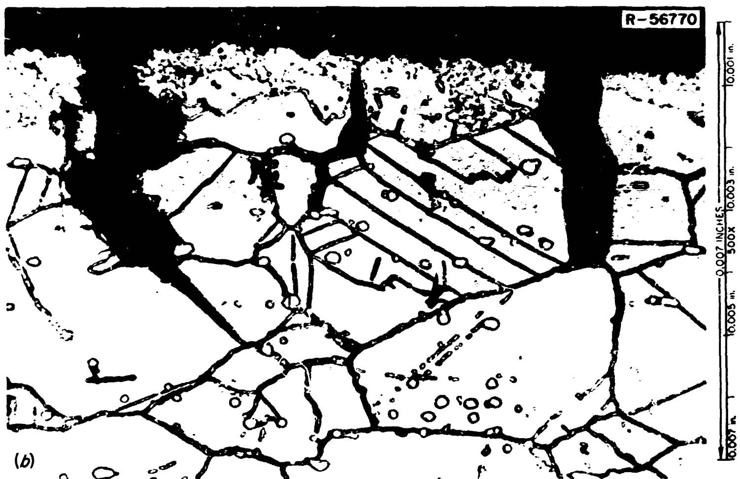
Fig. 97. Photomicrographs of the Tension Side Near the Fracture of a Bend Specimen from the Outside Liquid Region of the Mist Shield. (a) 100x. (b) 500x. Etchant: lactic acid, \text{HNO}_3 , \text{HCl} .
