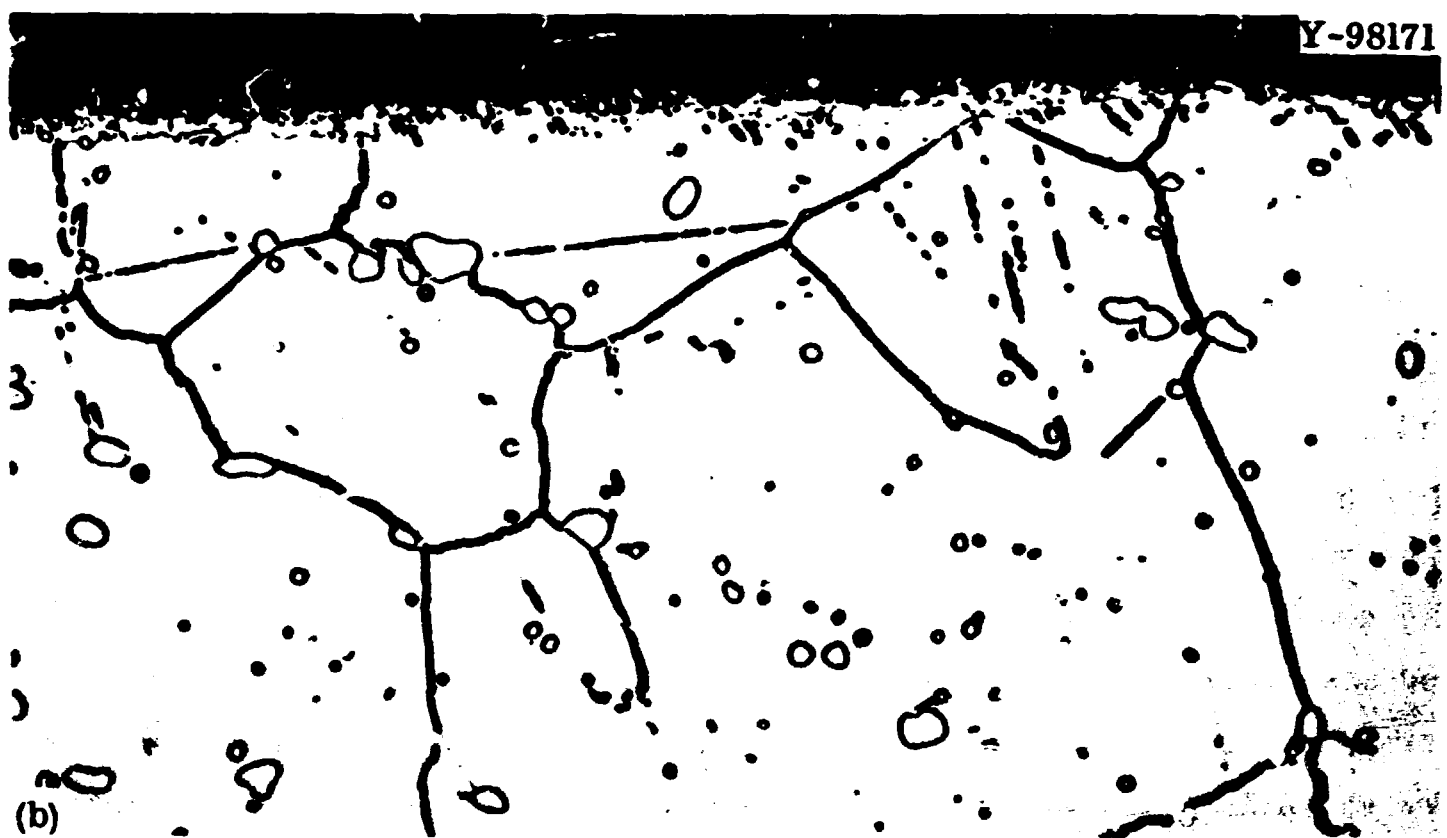
Fig. 36. Typical Photomicrographs of Heat 5085 After Exposure to Static Unenriched Fuel Salt for 19,136 hr above 500°C. 500 \times . (a) As polished. (b) Etchant: glyceria regia.
