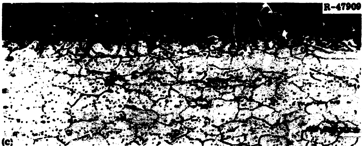
Fig. 24. Photomicrographs of INOR-8 (Heat 5065) Sample Exposed to Fluoride Salt in the HTR for 11,933 hr above 500°C and Then Tested at 25°C and a Strain Rate of 0.05/in. Thermal fluence was 9.4 \times 10^{20} neutrons/cm 2 . 100x. (a) Fracture, as polished. (b) Fracture, etched. (c) Edge of stressed portion. Etchant: aqua regia.
