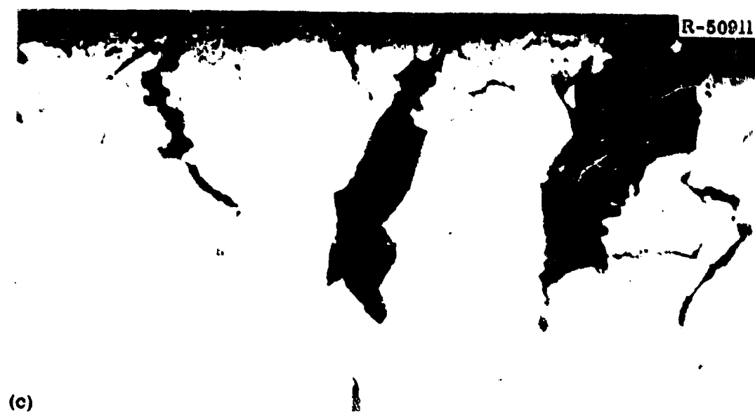
Fig. 44. Photomicrographs of INOR-8 (Heat 5065) Sample Tested at 25°C After Being Exposed to the MSRE Core for 19,136 hr Above 500°C and Irradiated to a Thermal Fluence of 1.5 \times 10^{21} neutrons/cm 2 . (a) Fracture, etched. 100x. (b) Edge, as polished. 100x. (c) Edge, as polished. 500x. (d) Edge, etched. 100x. Etchant: glyceria regia. Reduced 26%.
