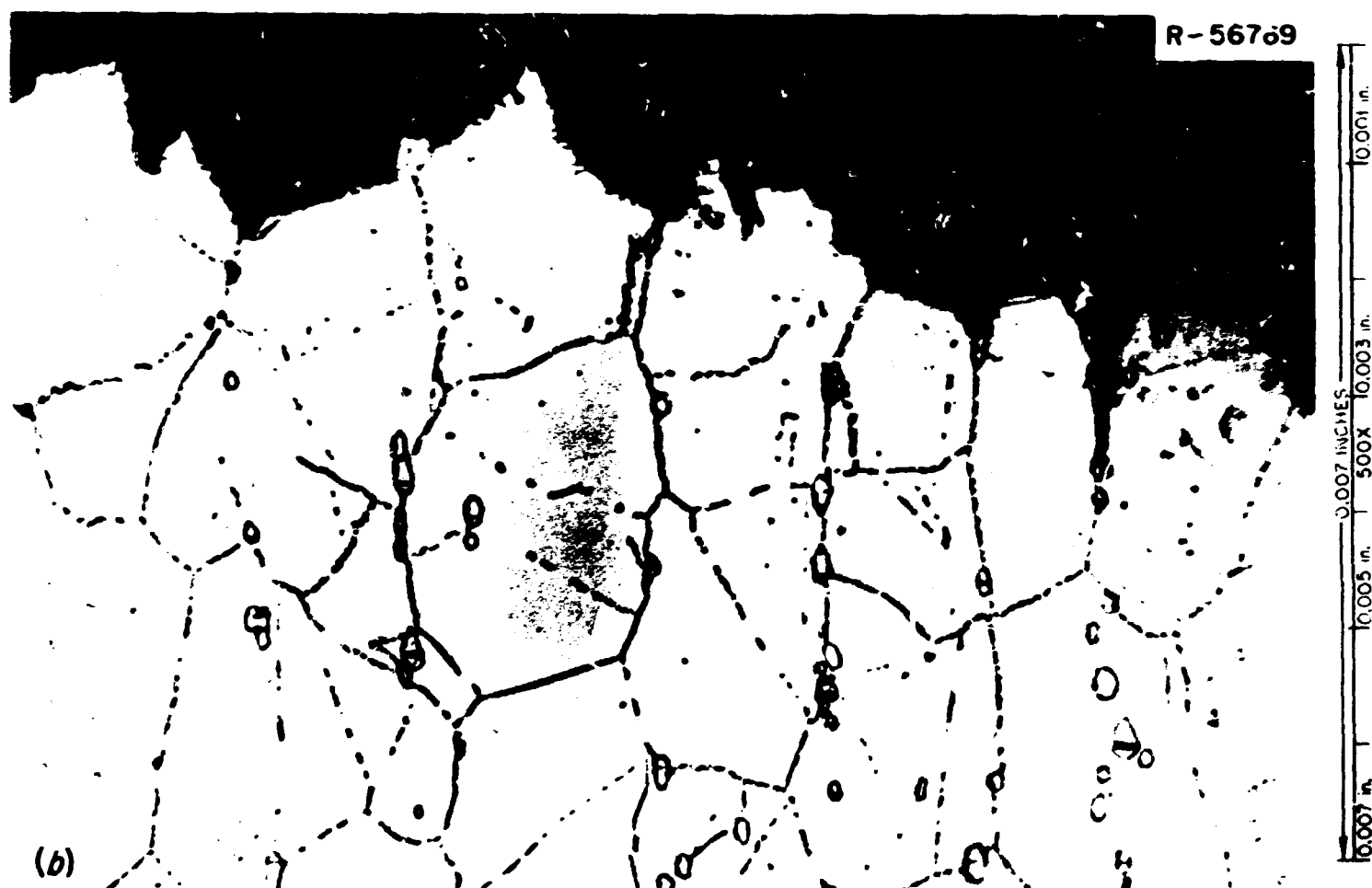
Fig. 96. Photomicrographs of the Fracture of a Bend Specimen from the Outside Liquid Region of the Mist Shield. (a) 100x. (b) 500x. Etchant: Lactic acid, \text{HNO}_3 , \text{HCl} .
