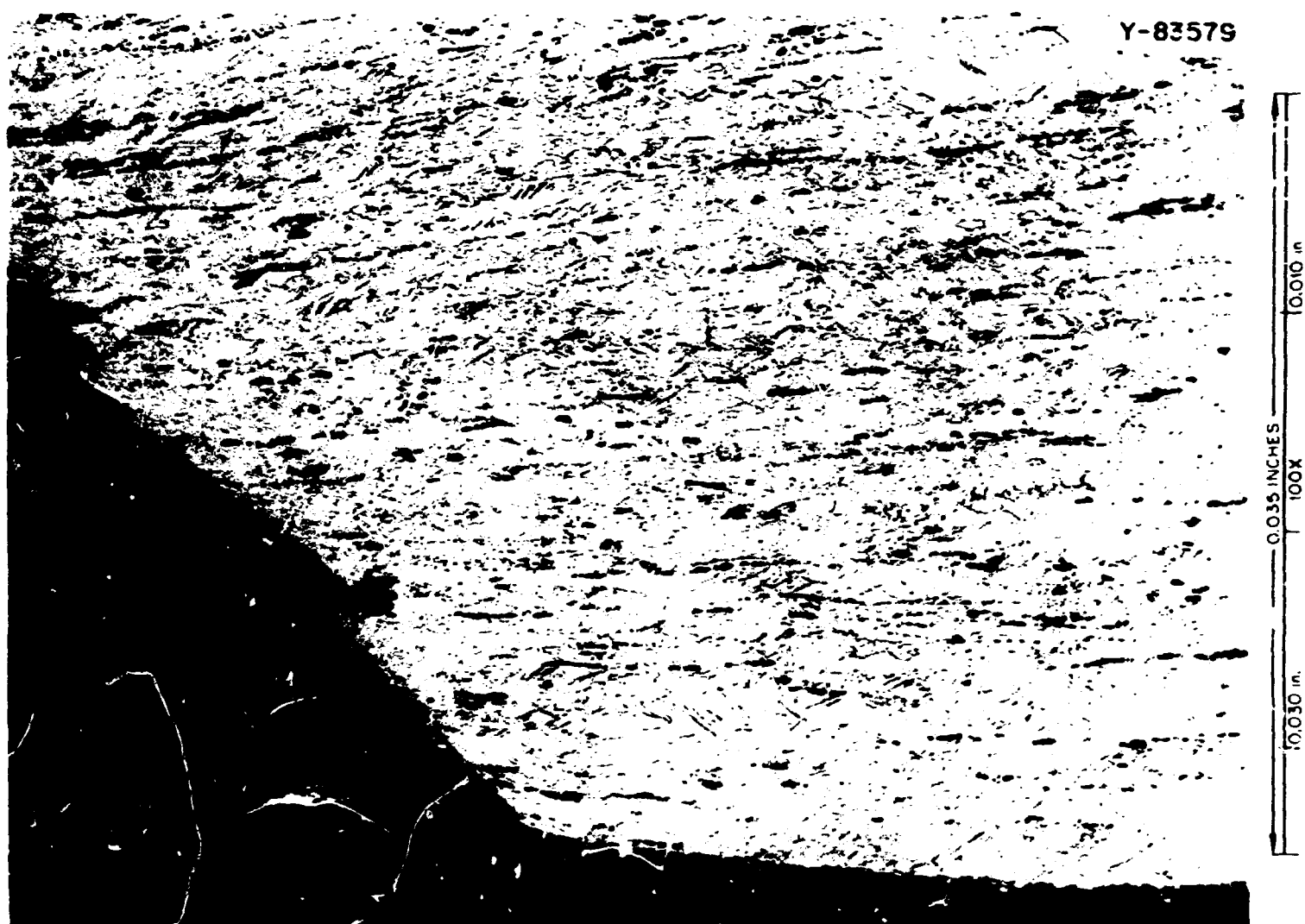
Fig. 15. Photomicrograph of the Fracture of a Zirconium-Modified INOR-8 Sample (Heat 21554) Tested at 25°C at a Strain Rate of 0.05/min. Exposed to a static fluoride salt for 5554 hr above 500°C before testing. Note the shear fracture and the absence of edge cracking. 100x. Etchant. glyceria regia.
