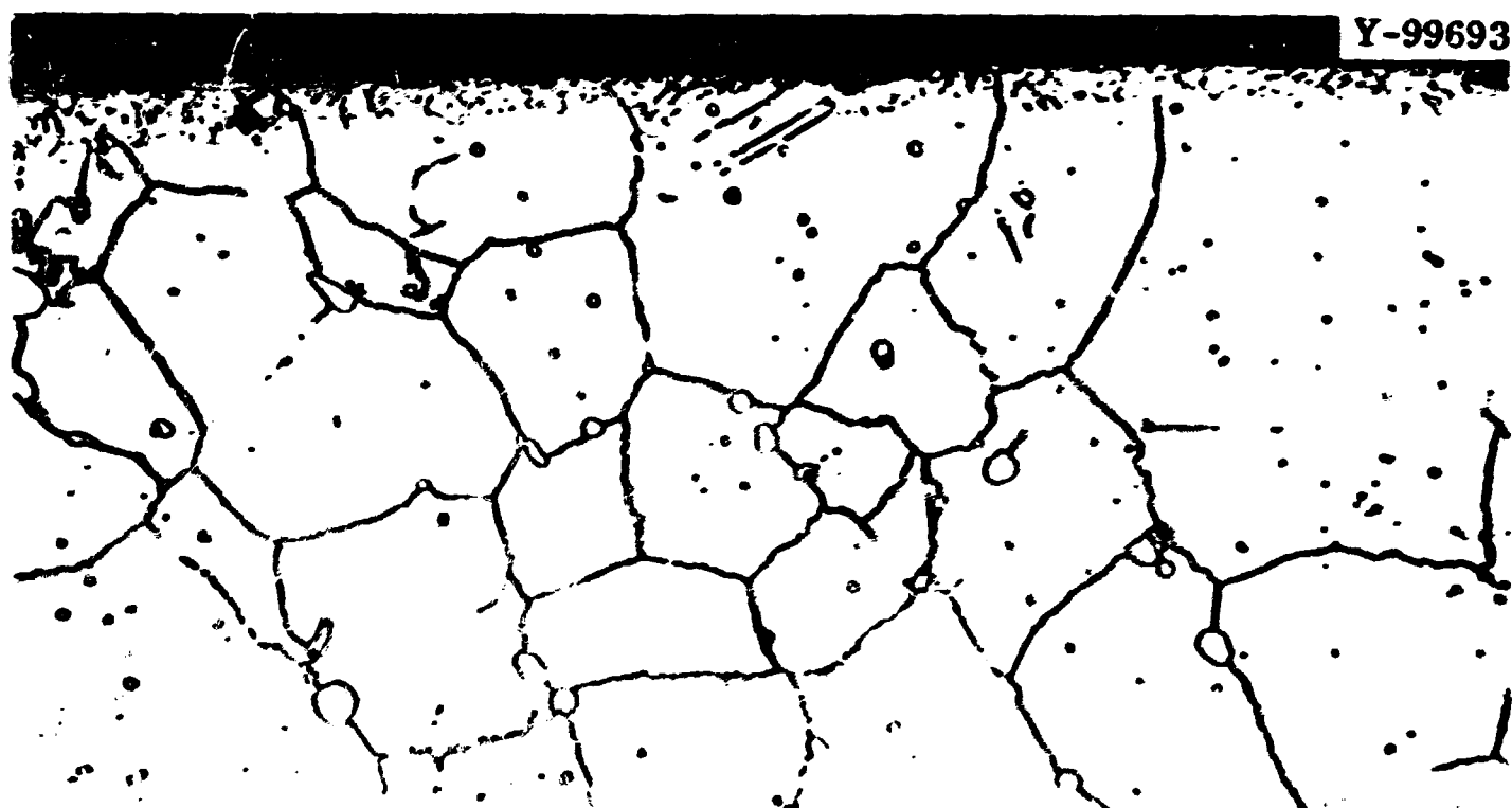
Fig. 58. Photomicrograph of INOR-8 (Heat 5085) Rod that was Annealed 1 hr at 1177°C, Centerless Ground 5.2 mils, and Annealed 4370 hr at 650°C in Argon. 500x. Etchant: glyceria regia.
