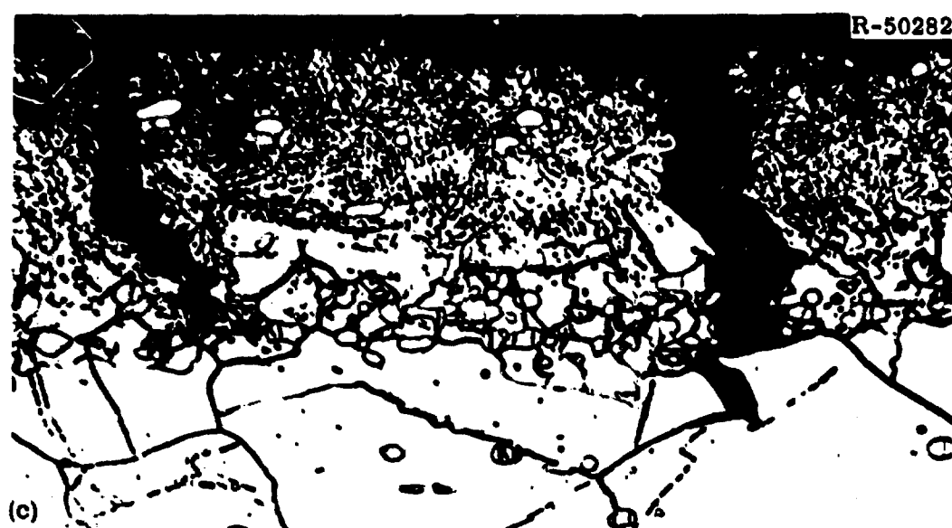
Fig. 49. Typical Photomicrographs of INOR-8 (Heat 5085) Sample Exposed to the MSRE Core for 19,136 hr Above 500°C. The sample was bent in a vise. (a) As polished, tension side. 100x. (b) As polished, tension side. 500x. (c) Etched, tension side. 500x. (d) Etched, compression side. 500x. Etchant: aqua regia. Reduced 27%.
