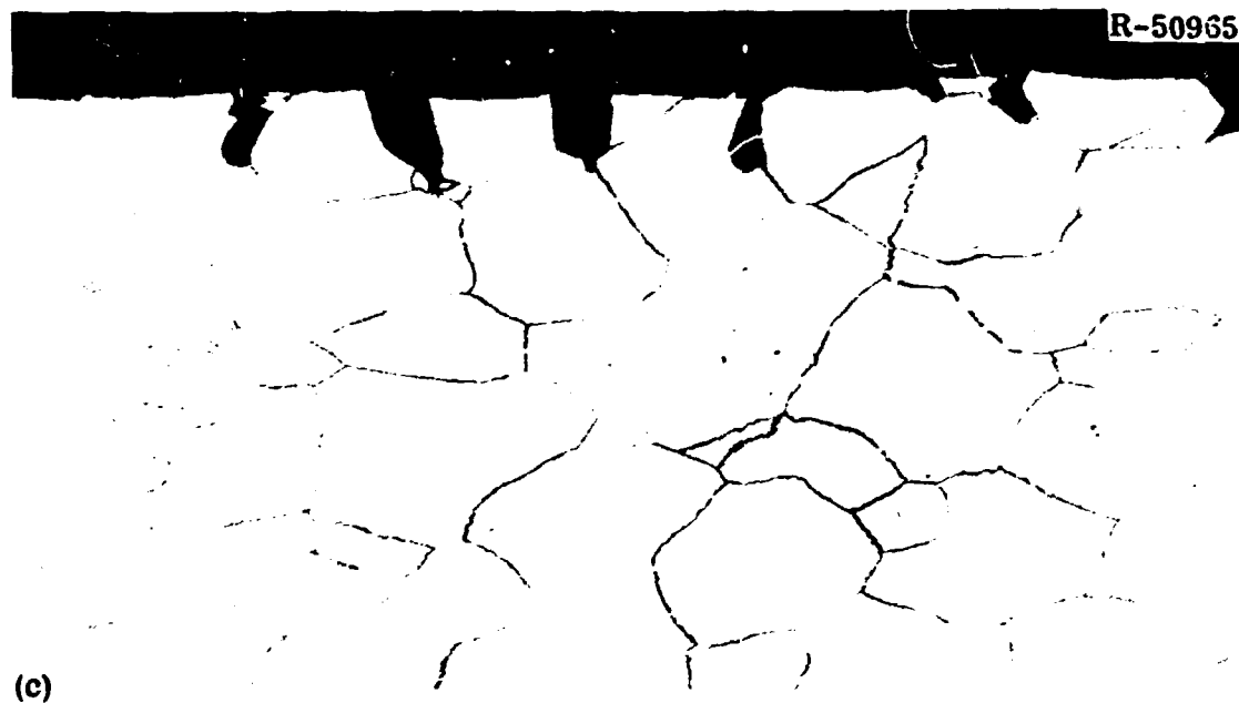
Fig. 51. Photomicrographs of a Modified INOR-8 (Heat 7320) Sample Tested at 25°C After Being Exposed to the MSRE Core for 7203 hr Above 500°C and Irradiated to a Fluence of 5.1 \times 10^{20} neutrons/cm 2 . (a) Fracture, etched, 100x. (b) Edge, as polished. 100x. (c) Edge, Etched. 100x. Etchant: glyceric acid. Reduced 22%.
