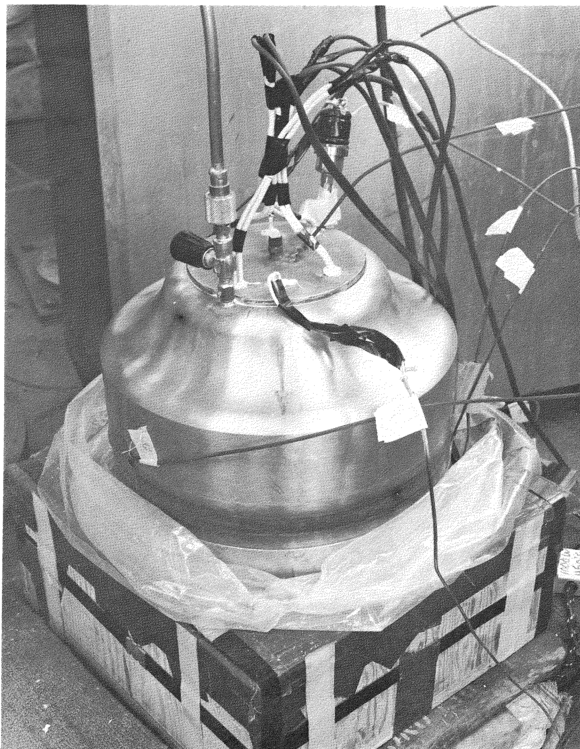
Figure 2-10. Unit 10D1 Instrumented for Thermal Test
