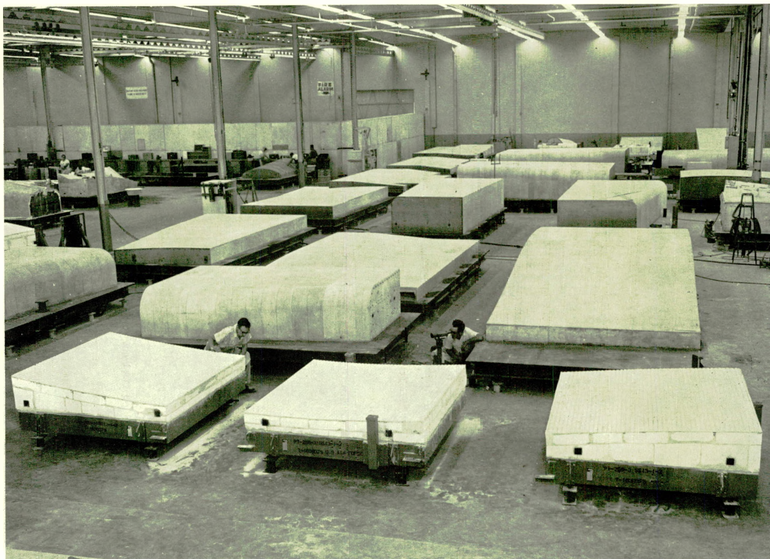
FIGURE 40. SIZE AND CONTOUR OF VARIOUS HONEYCOMB SANDWICH PARTS MADE FOR XB-70 ARE ILLUSTRATED BY THESE CERAMIC FACES FOR ELECTRIC BLANKET BRAZING (Ref. 78)
