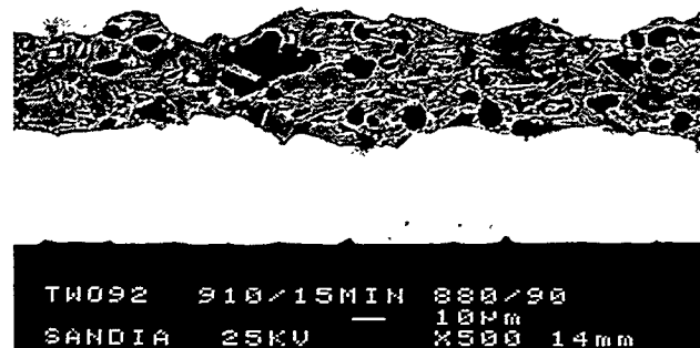
Figure 3-7. Time development of Ti_2O_3 /TIF containing core at 880°C.
