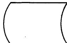
Drum, Disc, or Random Access unit (input or output)
