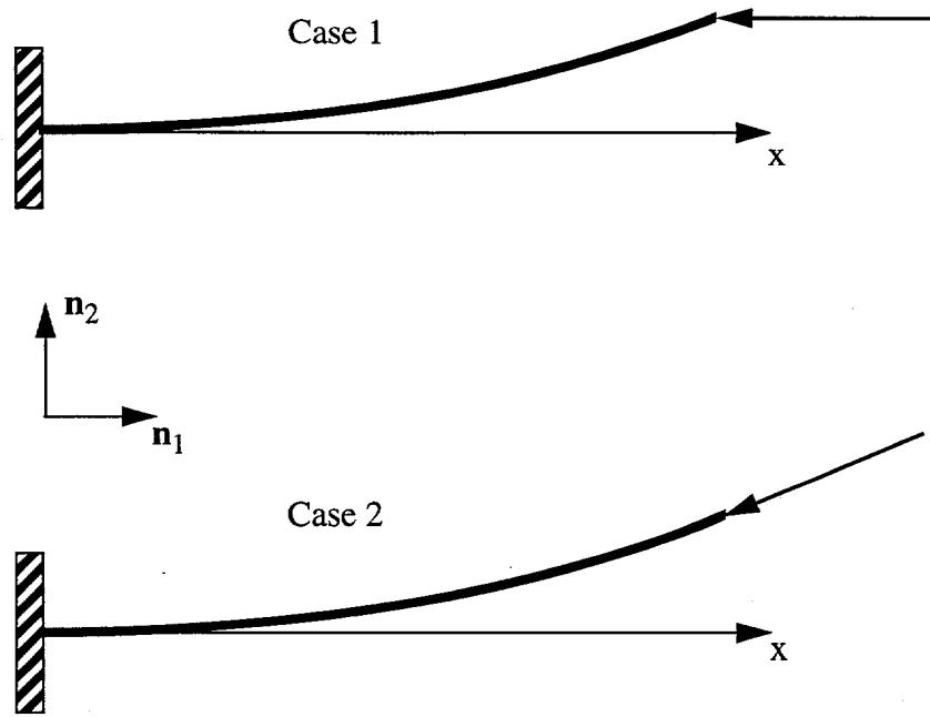
Figure 1: Load cases for cantilevered beam example.
