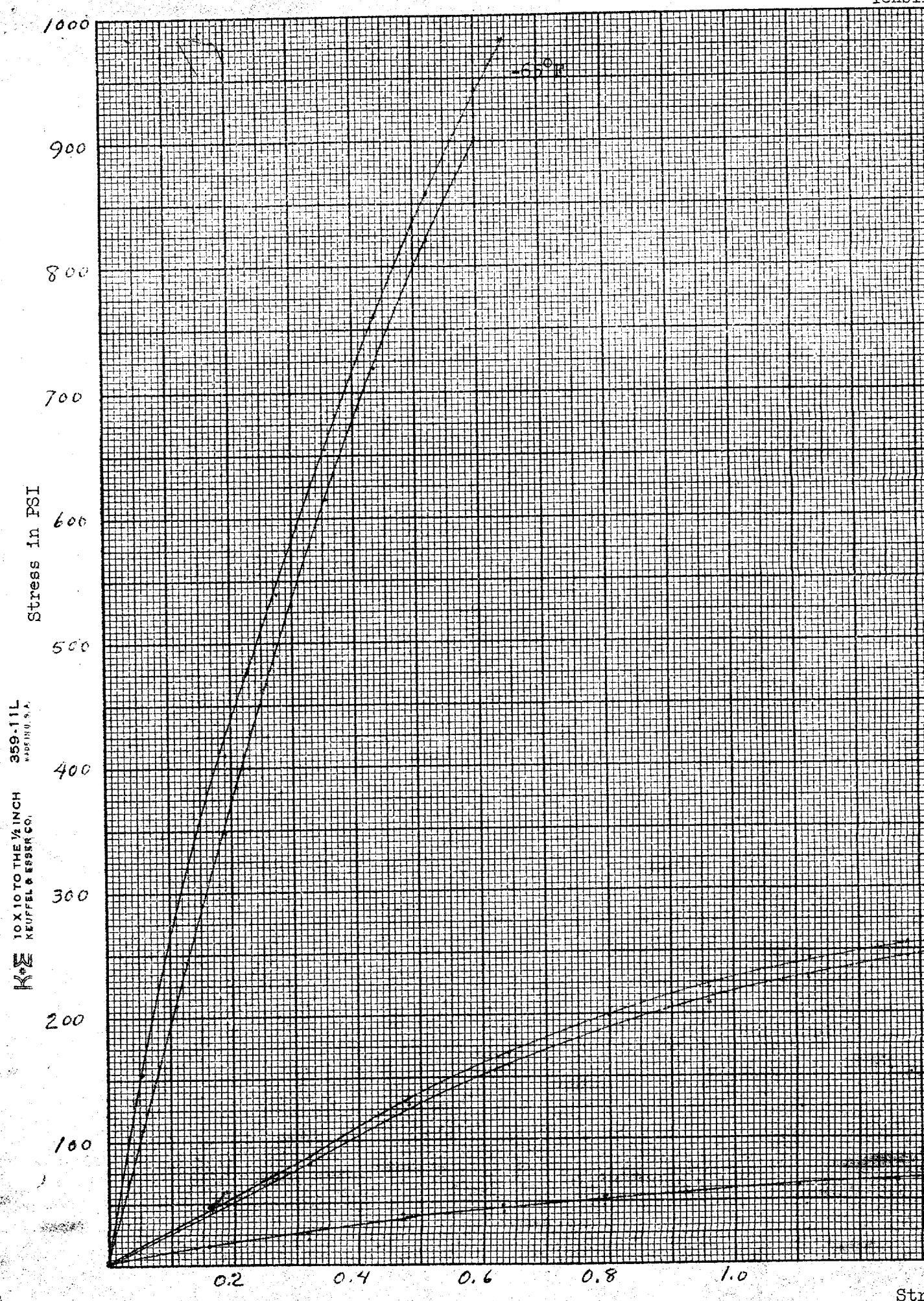
Tests - LX-03-0 with 90° Adiprene Glue Joint,
