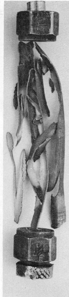
Figure 39. Typical Annealed Zircaloy-4 Burst-Test Specimens Showing Modes of Fracture
