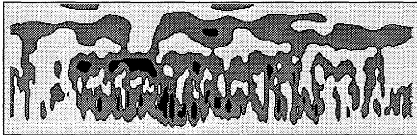
Figure 7. Gauss-Hermite transform of about one-tenth sec of a noisy audio tape, sampled at 22050 Hz. The scale ranges from about 0.14 ms at the bottom to about 5.7 ms at the top. The transform was computed with derivative order 10 to enhance the coherence of events that last longer than the background noise; p was set to 1.4 to emphasize the smaller scales; the frequency range is from 100 Hz to 3200 Hz; and the scale spans a little over 5 octaves with 12 voices in each octave.
