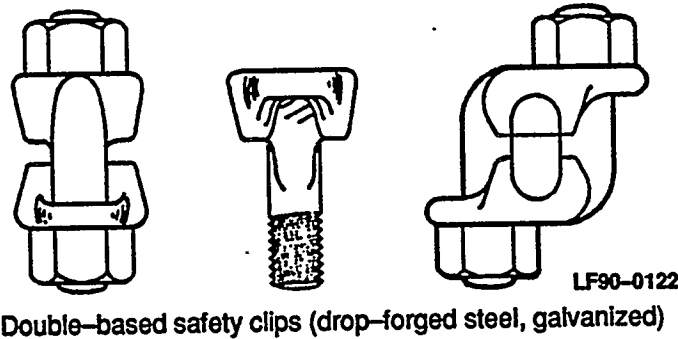
Figure 8-13. Double-based safety clips (drop-forged steel, galvanized).
