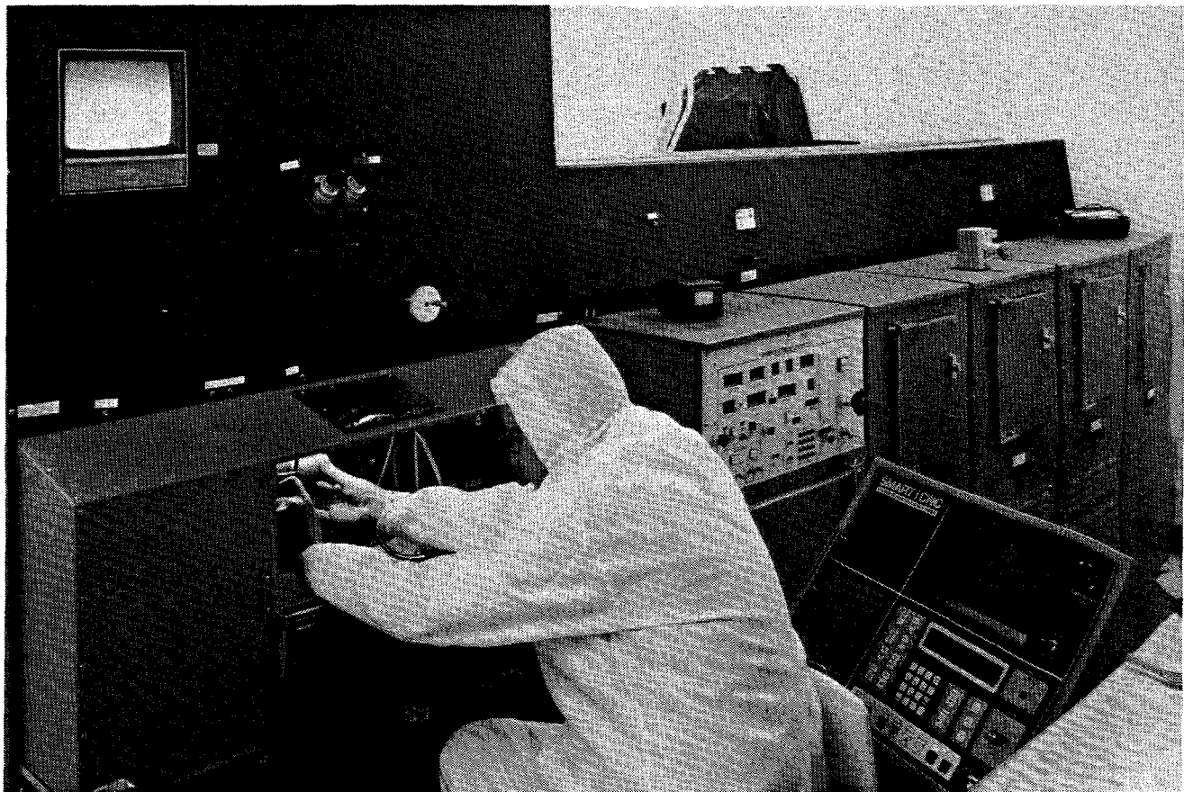
Laser welder operator loads a component into the fixture in preparation for welding.
