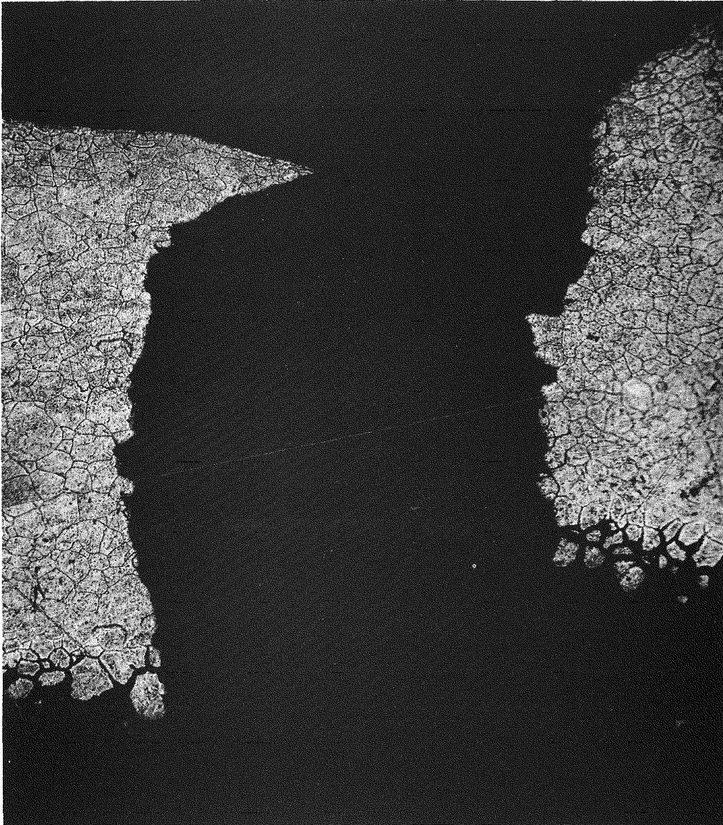
Fig. 5.1 Fracture region of GB-9 cladding burst-test sample showing intergranular failure to ~80% of cladding and transgranular failure through remainder
