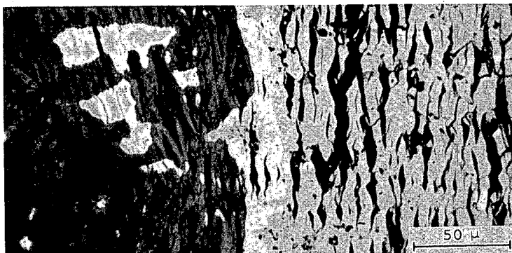
Figure 29 (R-27-B8) As Polished X_2 phase and white phase layer at the center of the fuel. Dark final corrosion product con- taining particles of the white phase and X_2 phase.
