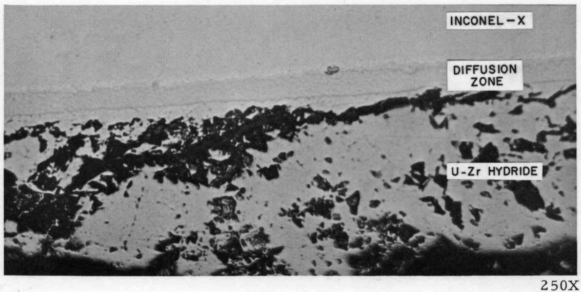
Figure 5. Inconel-X vs U-Zr Hydride — 216 Hr at 1200°F
