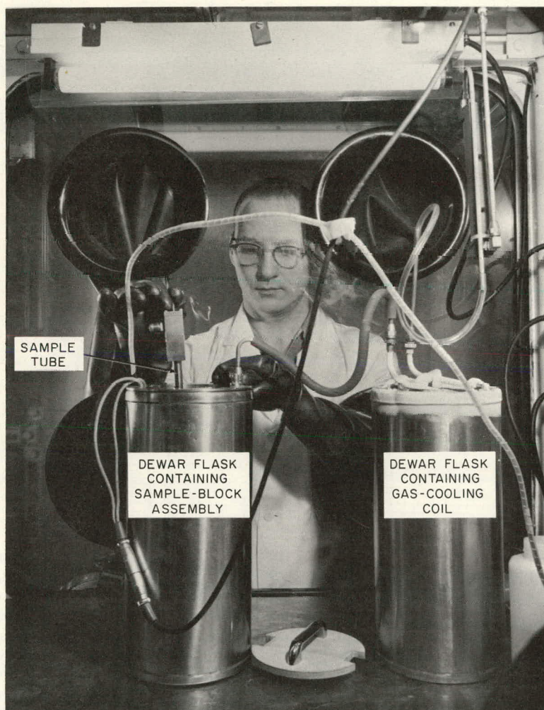
Fig. 7. Operation of Thermal-analysis Apparatus; Placing a Sample Tube into Sample-block Assembly
