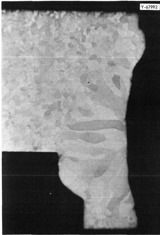
Fig. 33.2. Section of Electron-Beam Weld in W-2% Mo Alloy. 16 \times . Notice the larger grain size but absence of porosity and weld metal overhang. Reduced 25%.
