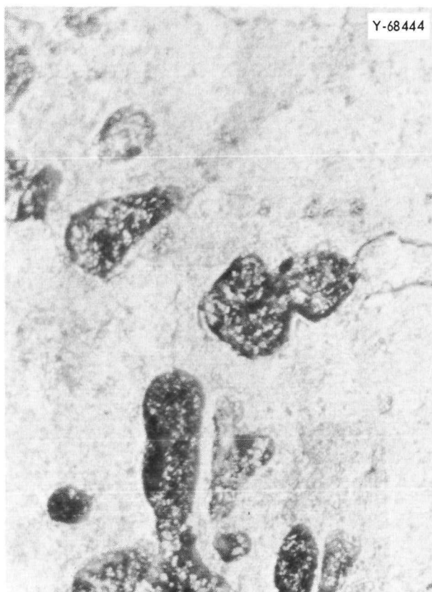
Fig. 37.2. Microstructure of Hypereutectic Pb-0.9% Li Alloy.
