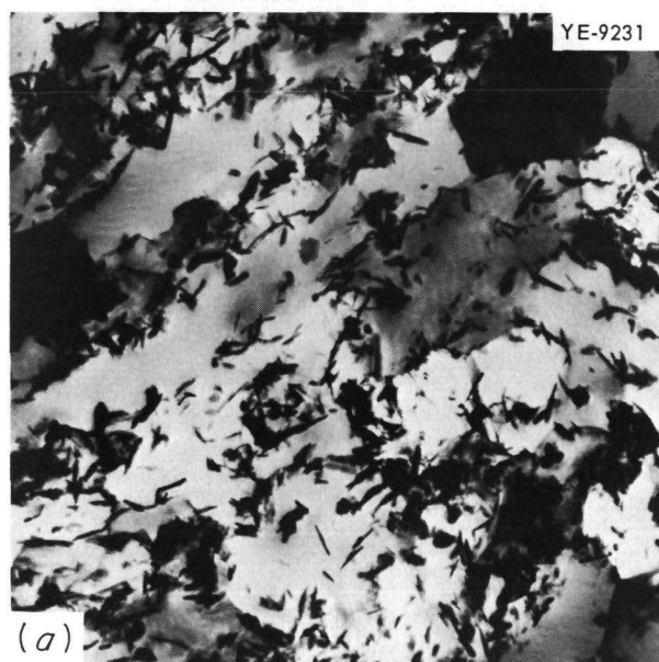
Fig. 22.2. Microstructures of Sintered Aluminum Products. (a) ORNL material containing 6% \text{Al}_2\text{O}_3 . 21,000 \times . (b) Commercially produced material containing 7.8% \text{Al}_2\text{O}_3 . 18,000 \times .
