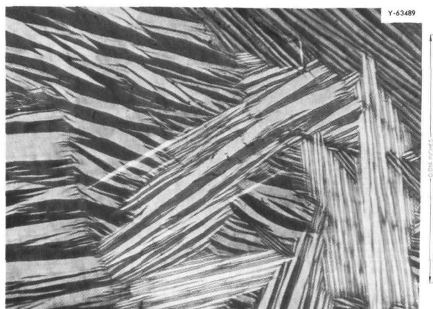
Fig. 34.4. Microstructure of Cerium Dicarbide Under Polarized Light. Etched electrolytically with equal parts concd lactic, acetic, and sulfuric acids. 250 \times . Reduced 48%.
