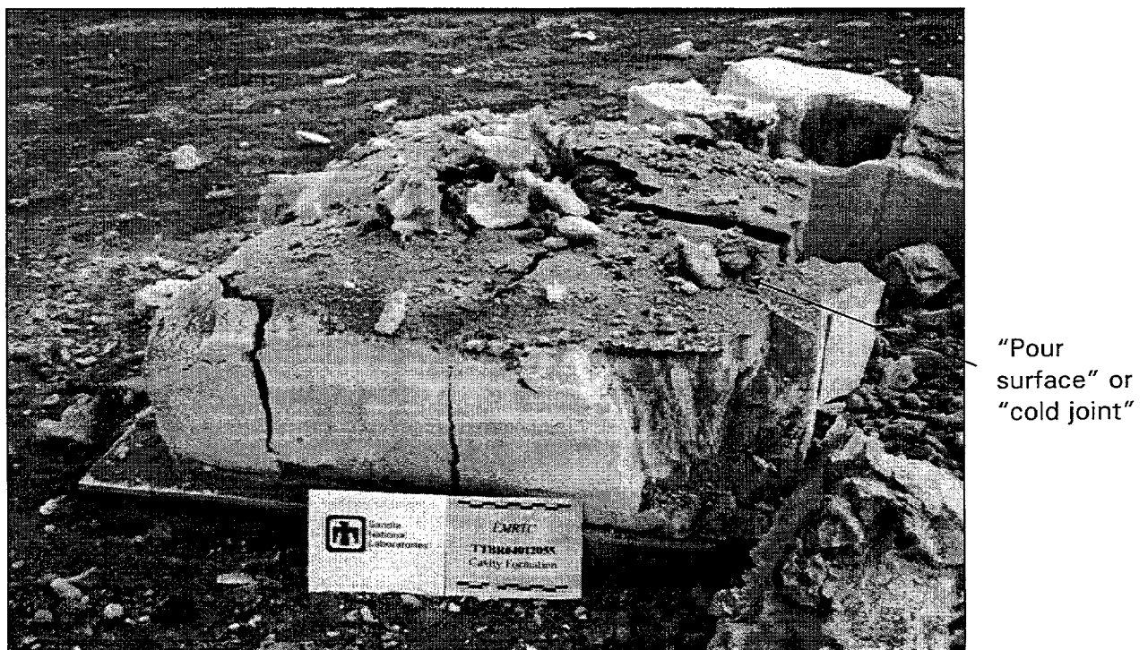
Figure 38. Block #04-02 following 100 gm C-4 Embedded Shot
