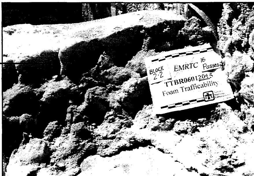
Figure 66. Block #02-02 After 16 Passes by M110 (pads on at low speed)
