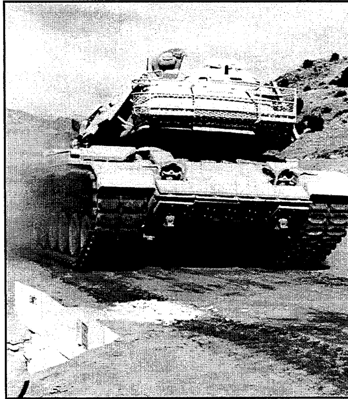
Figure 63. M60 Tank in a High-Speed Run over 4 pcf Foam (the right-hand track relative to the driver, left in photo, has road pads; left-hand track is "bare")
