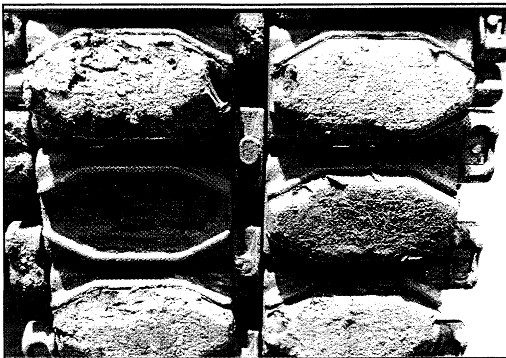
Figure 55. M60 Track with One Road Pad (center left) Removed
