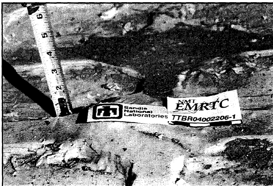
Figure 77. Rut in 6 pcf Foam ( \frac{1}{2} inch after several passes)
