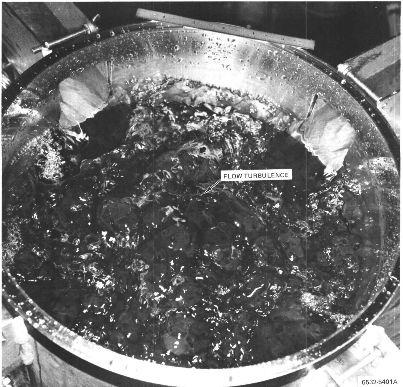
Figure 27. SPF Model Flow Conditions without Baffles or Diffusers
