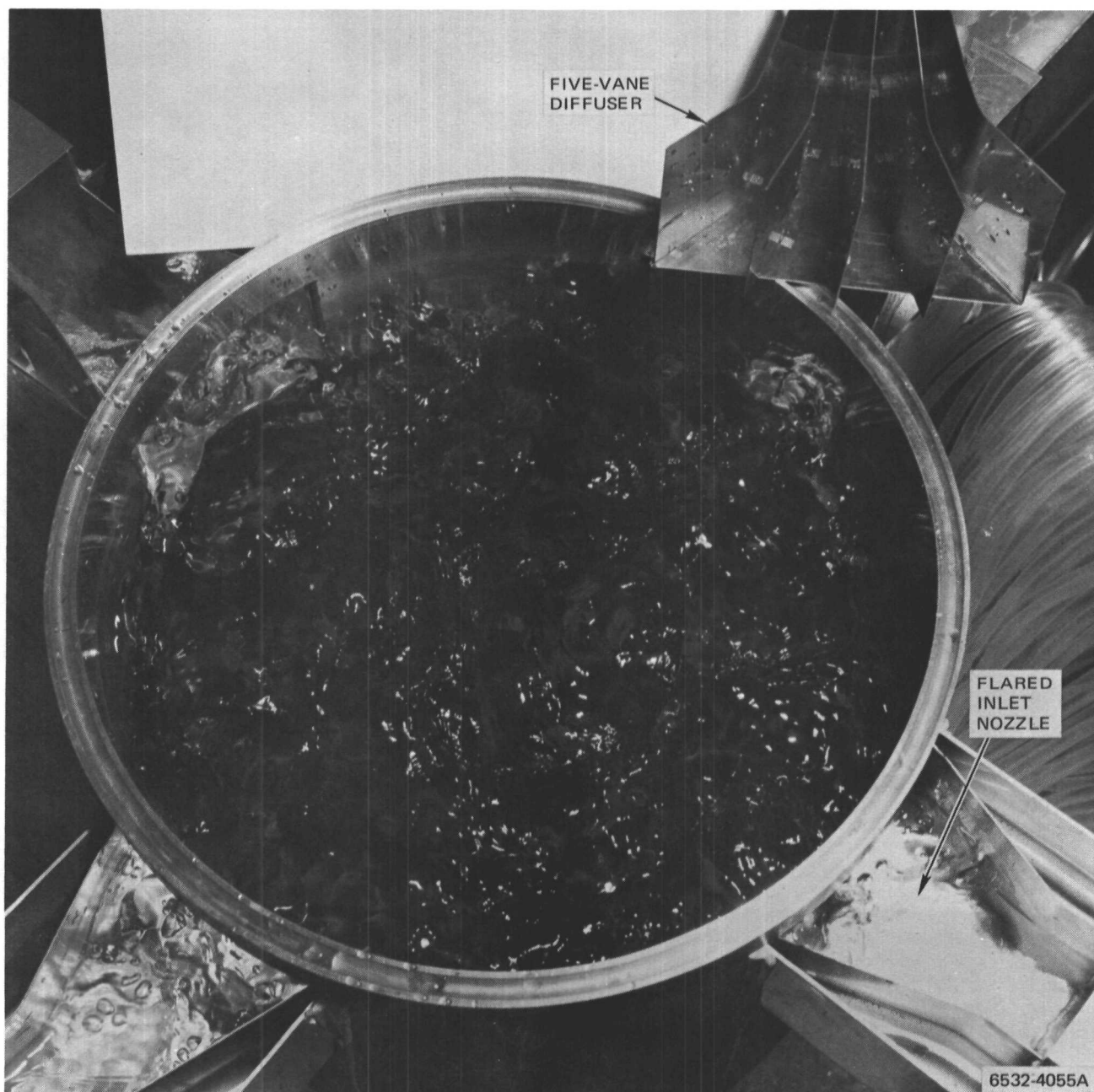
Figure 26. SPF Model with Straight Flared Inlet
