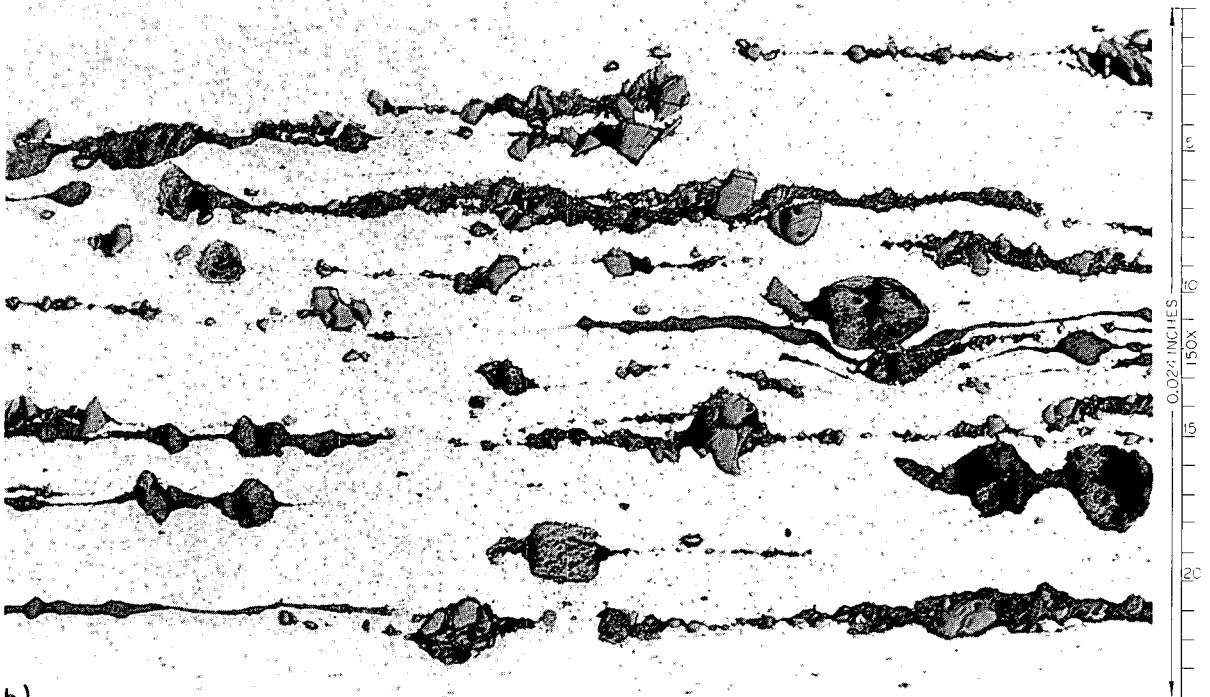
Fig. 7. Longitudinal Views of the D Oxide in Rolled Plates. Unetched. (a) Plate C-11-D, schedule A. (b) Plate C-5-D, schedule B.
