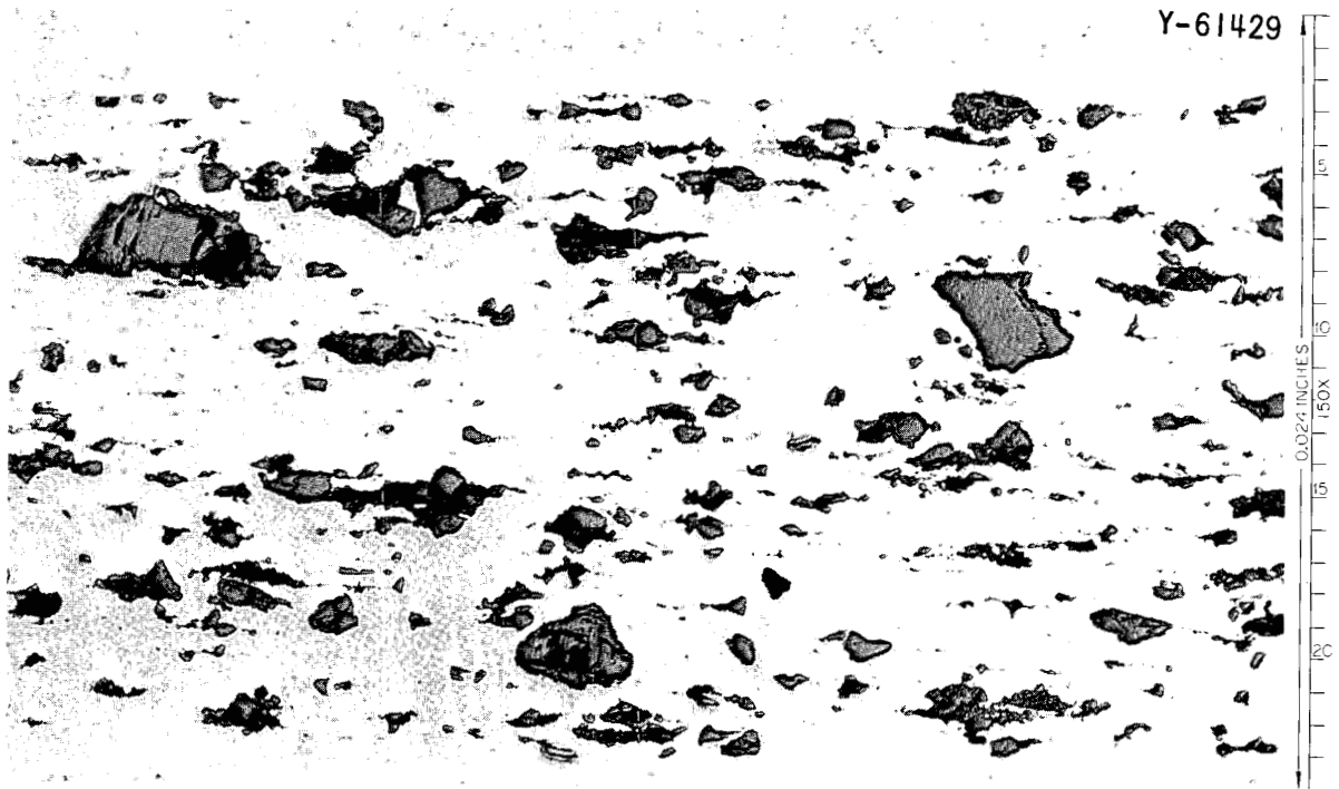
Fig. 8. Transverse View of a Straight-Rolled (Schedule A) Plate Containing S Oxide.
