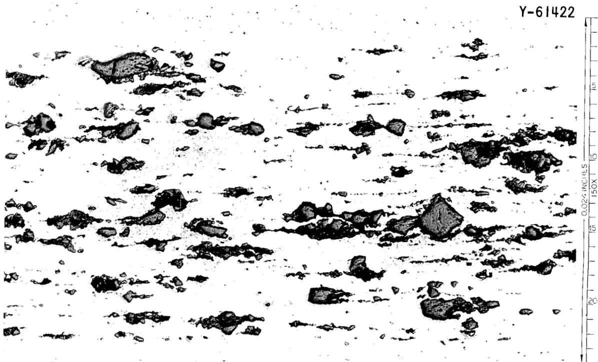
Fig. 9. Transverse View of a Cross-Rolled (Schedule B) Plate Containing S Oxide.
