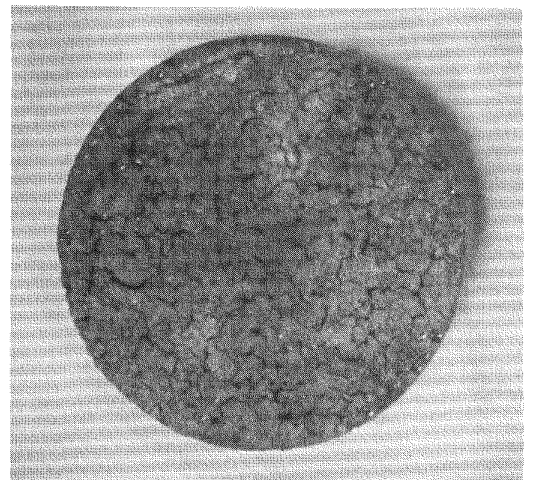
Fig. 9-36. Fuel rod 4C-153 before and after irradiation in capsule HRB-5 to 1.1 \times 10^{21} n/cm 2 at 1250°C (design). Rod 4C-153 was fabricated by the admix-compaction process using uncoated RC4 shim and isotropic graphite filler and was high-fired in H-327 graphite tubes to simulate in-block curing. This rod contained TRISO UC 2 (resin) fissile, BISO ThO 2 fertile, and BISO carbon inert particles.
