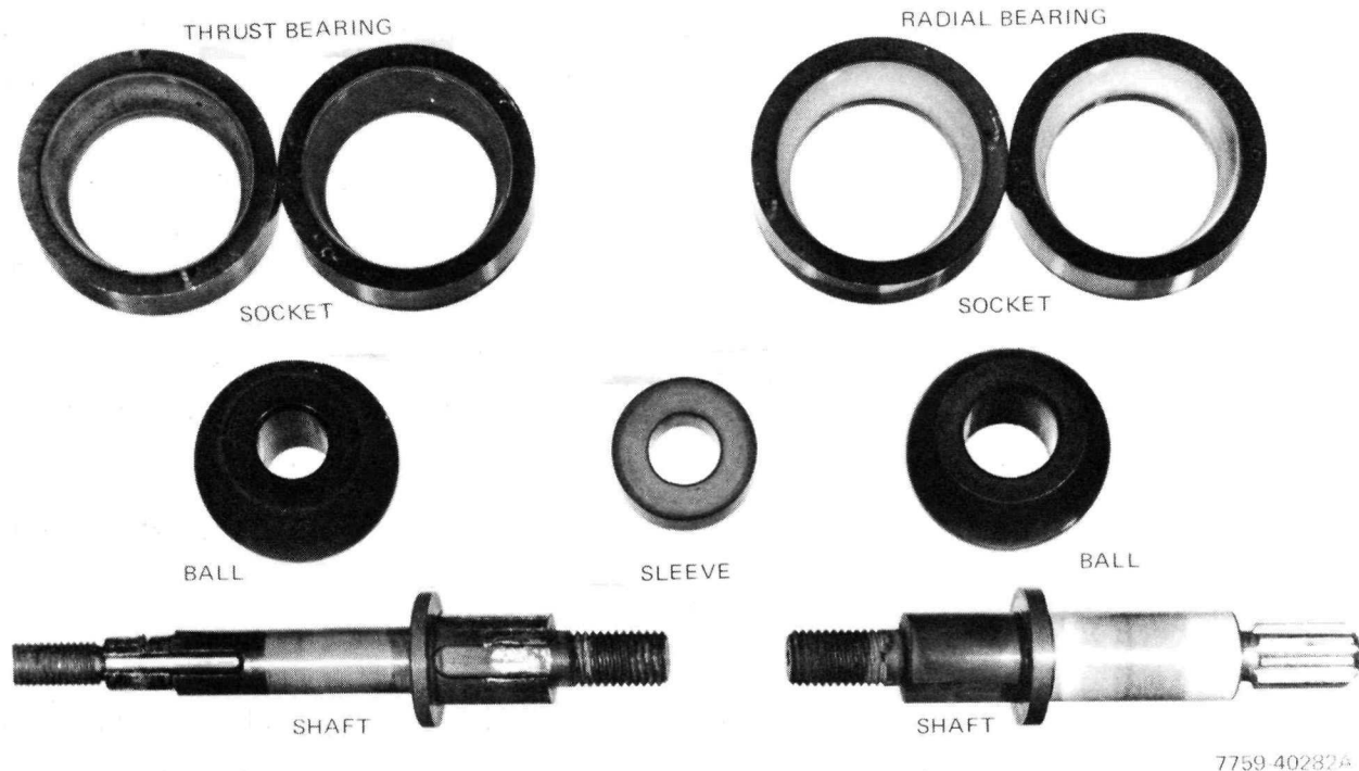
Figure 32. Post-Test Condition of S8DR Design Verification Bearing, Test 1 (Reference Bearing)
