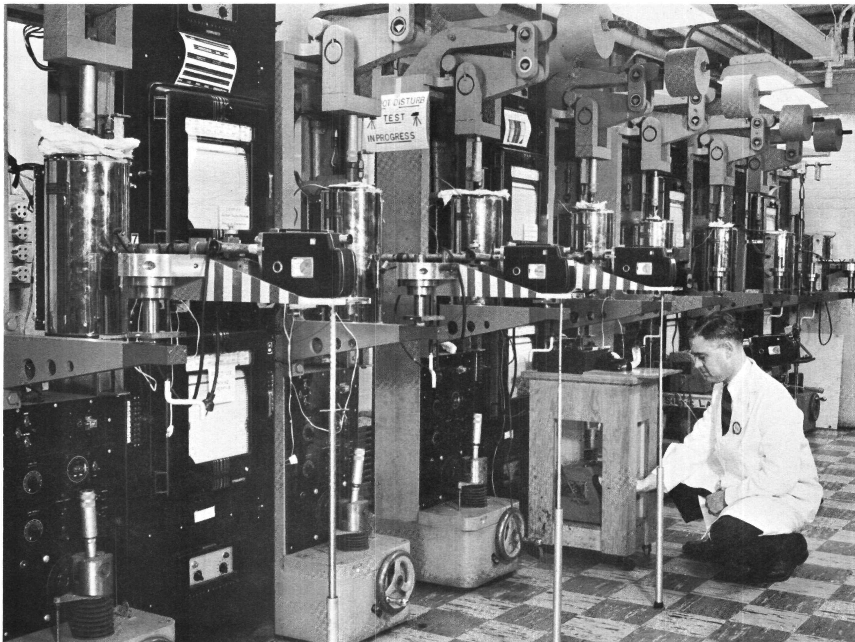
Fig. 15. Test Facility Used for Creep Measurements
