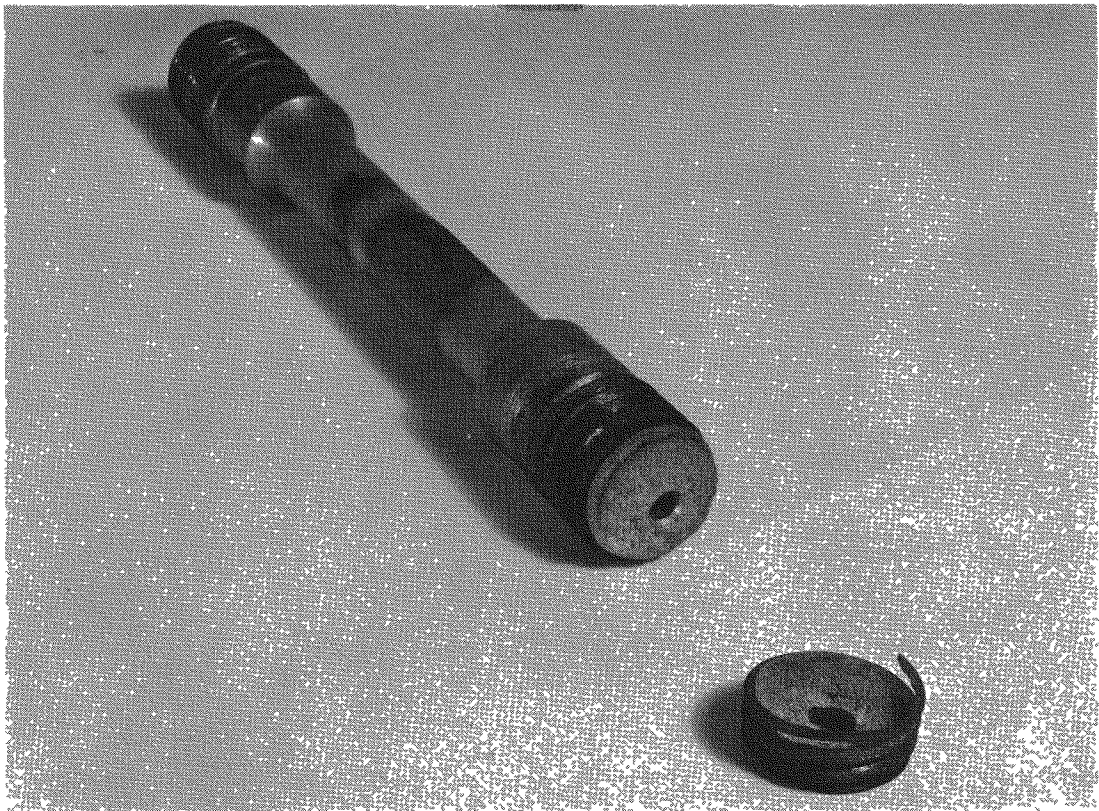
Fig. 23. Creep Test Specimen that Failed Before Load Application
