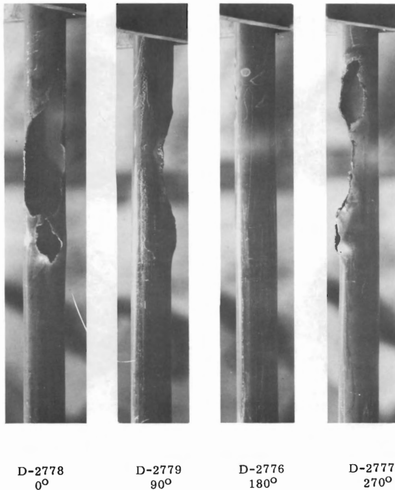
FIGURE 9. Cladding Rupture in a Vibrationally Compacted UO_2 -4 wt% PuO_2 PRTR Fuel Rod. Rupture Occurred in the Area of the Rod Previously Defected with a 1/16 in. diam Hole.
