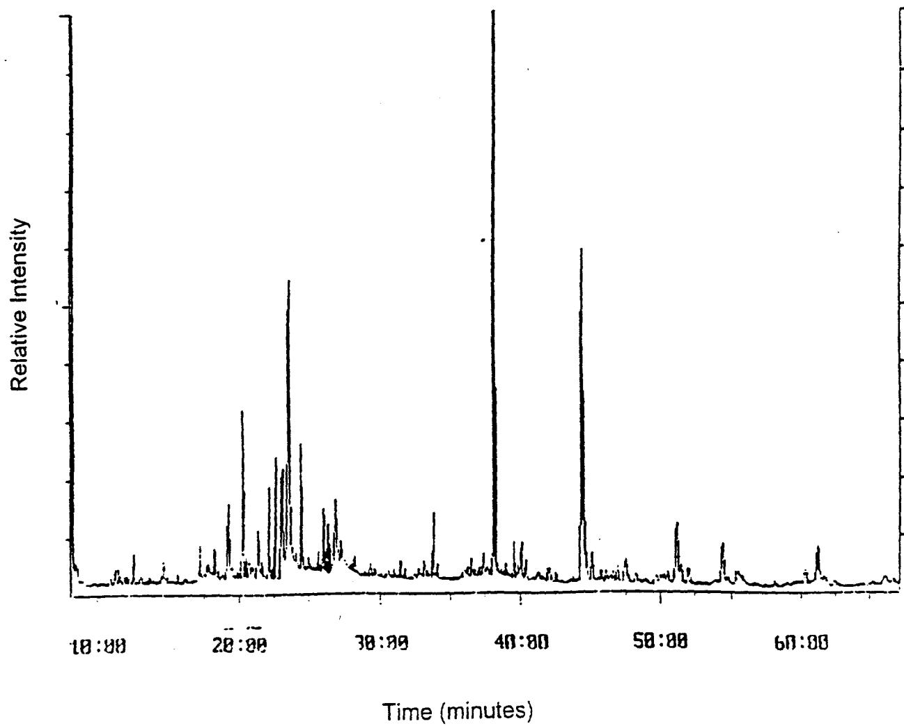
Figure 2. Total ion chromatographic profile of fingertip extract from adult male. Peaks at approximately 38 and 45 minutes are squalene and cholesterol, respectively.
