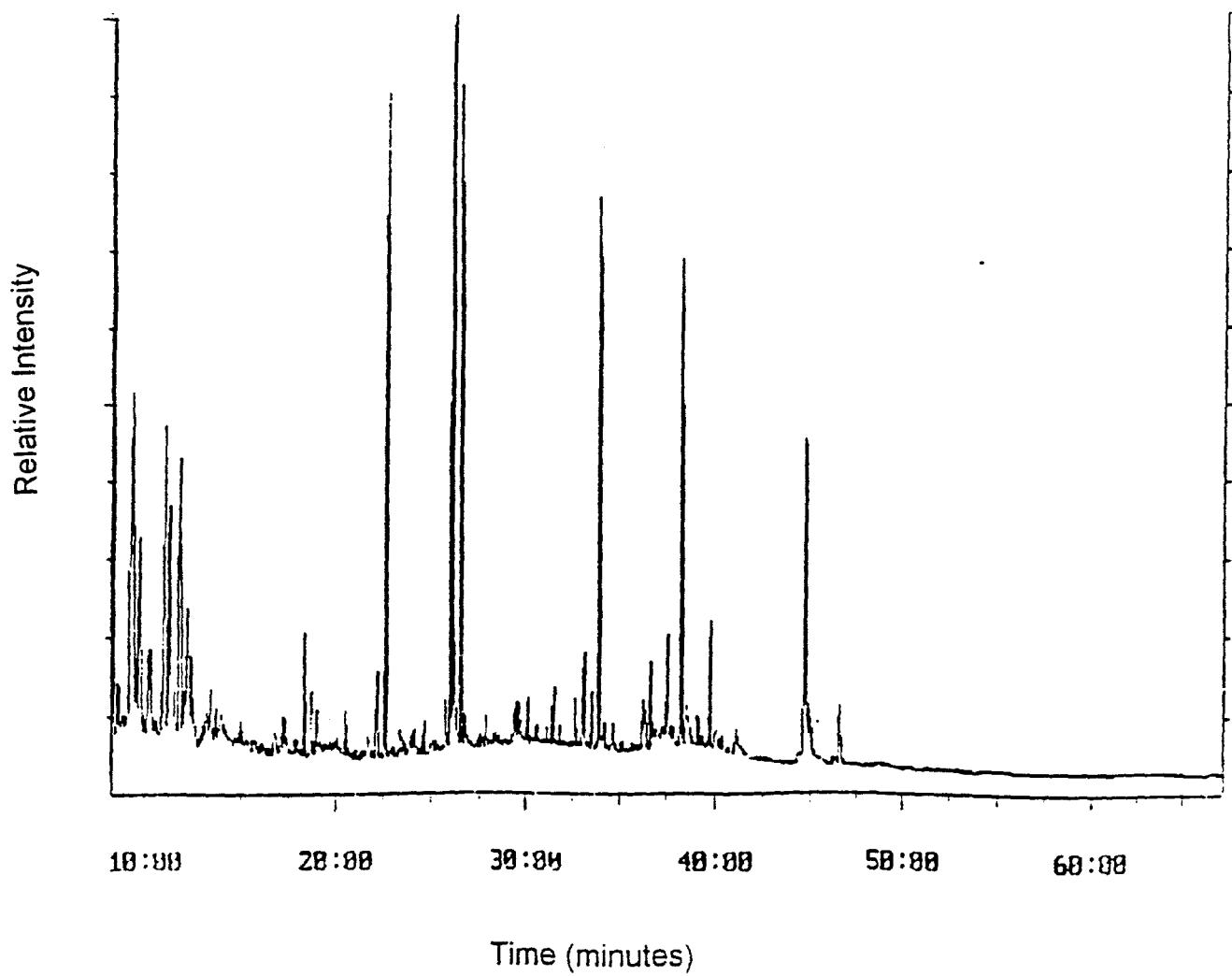
Figure 1. Total ion chromatographic profile of fingertip extract from four year old male. Peaks at approximately 38, 45 and 47 minutes are squalene, cholesterol, and an isomer of cholesterol acetate, respectively.
