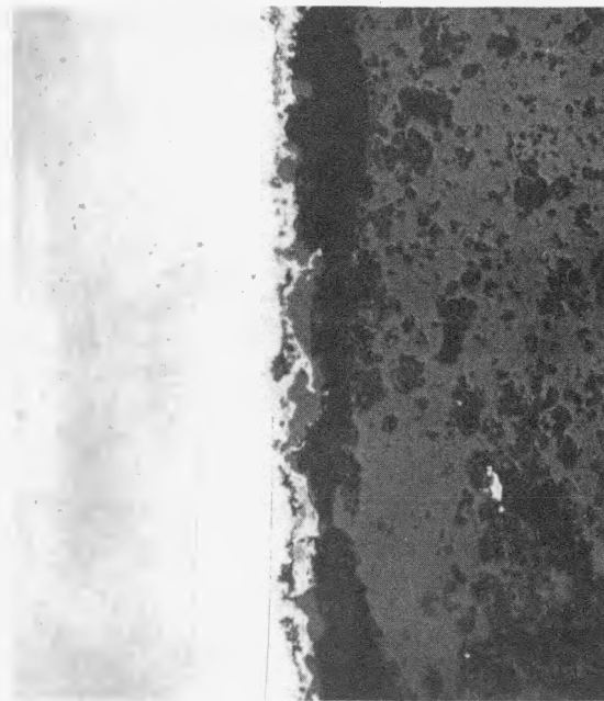
Fig. 5.3 Typical cladding attack in the top longitudinal section of fuel column in capsule G-3
