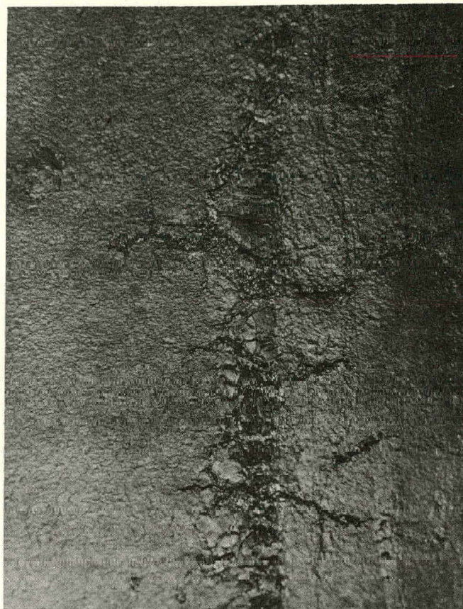
Figure 7. Photomicrograph Showing a Region of Surface of the Ingot in Figure 6. The foreign material is part of the 304 stainless steel can which has bonded into a defect in the sheet during rolling. 3X
