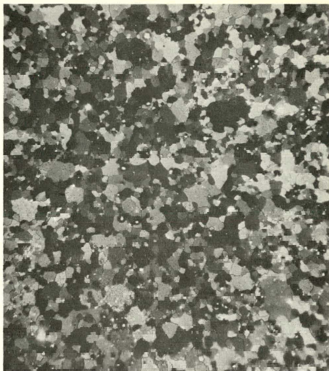
Figure 11. Photomicrograph of 0.1-in.-thick Ingot-Sheet Material that has been given by Eleven Passes at 1400°F. Polarized light. 50X
