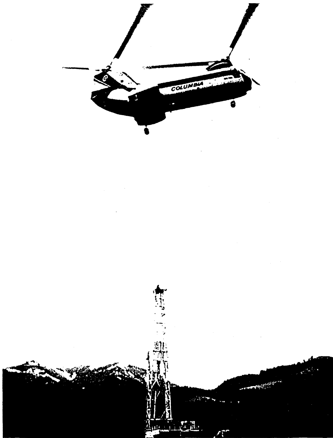
Figure 20. Boeing Vertol 107-II used to drill the BLM well in Wyoming (Courtesy of Columbia Helicopters).
