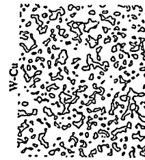
Continuous Area - Tungsten Dispersed Area - Copper
