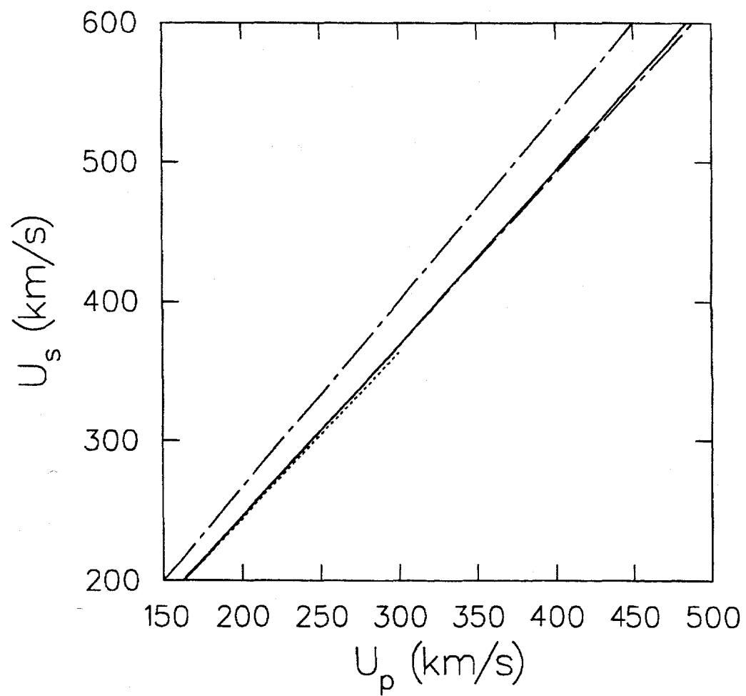
Fig. 2. Mo Hugoniot— $U_p$  out through turnaround. The dashed line is from the fit above the break. It shows that the straightness of the solid Hugoniot curve persists to quite high  $U_p$ .
