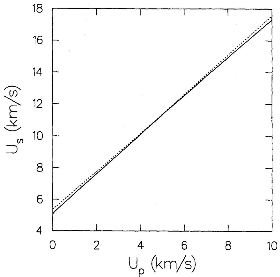
Fig. 1. Mo Hugoniot—lower portion around break. The solid line is the Mo Hugoniot. The two dashed lines are straight line fits to the two linear portions of the Hugoniot. (The dashed lines might appear to the eye as one straight line since their slopes are almost the same. Their intersection is around 5 km/s.)
