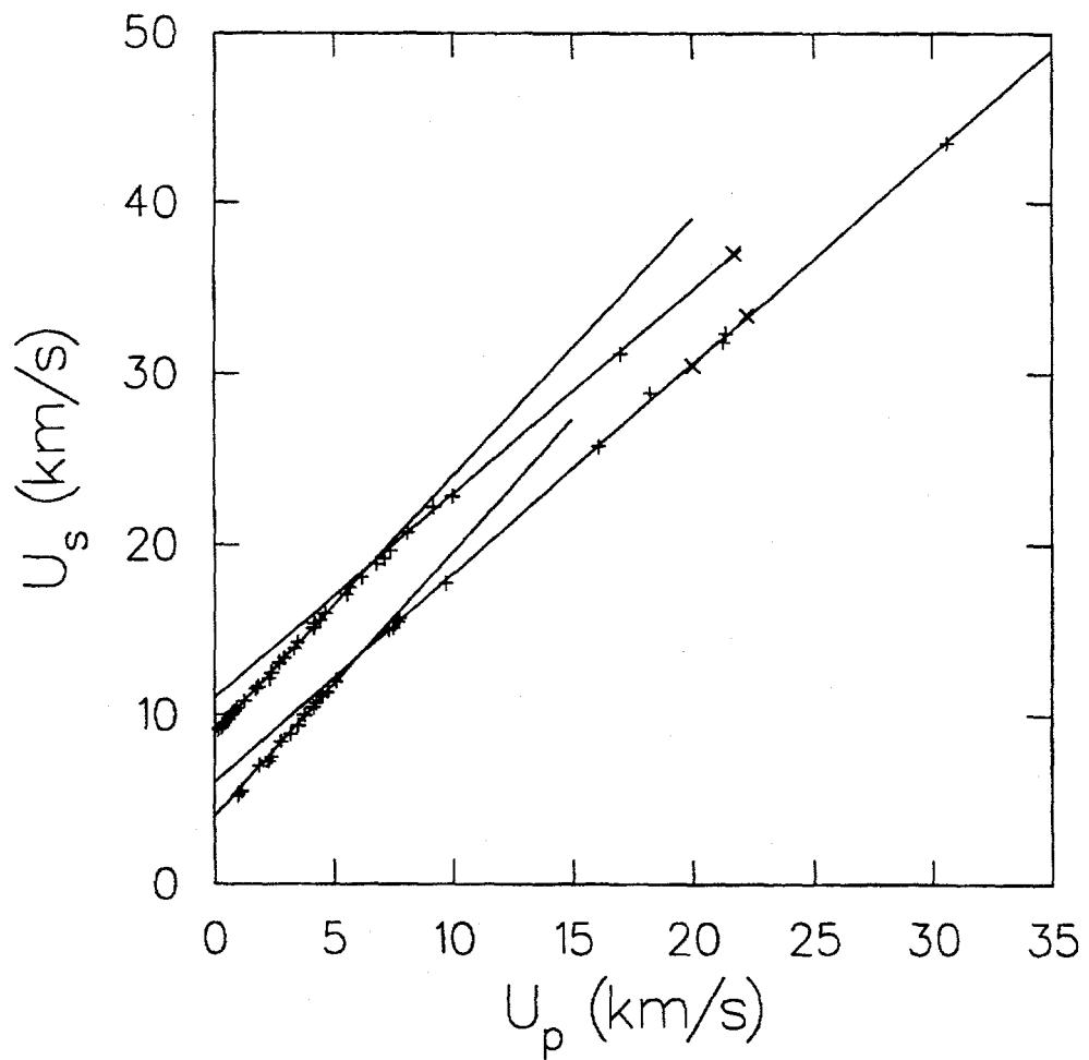
Fig. 3. Fe and Cu Hugoniot data. We see clearly the linearity of the upper data and a well-defined break. The Cu data and curves have been shifted upwards.
