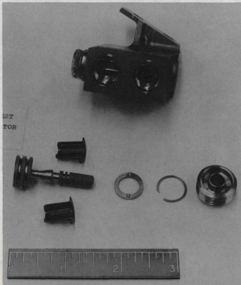
Figure 53. Drum Release Actuator, Disassembled
