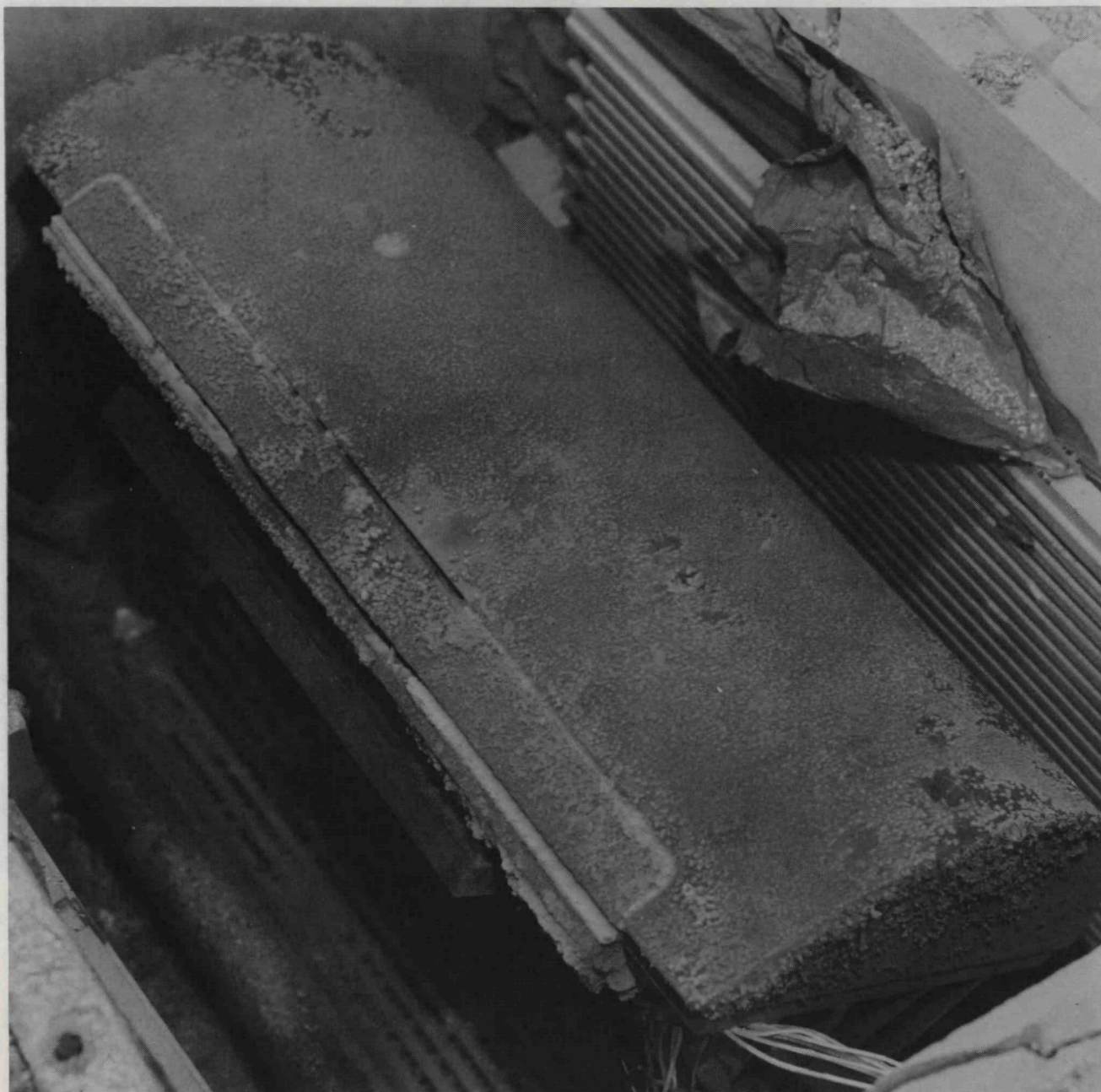
Figure 36. Post-Exposure Appearance of Be Control Drum at 1300° F for 300 Hours in Argon
