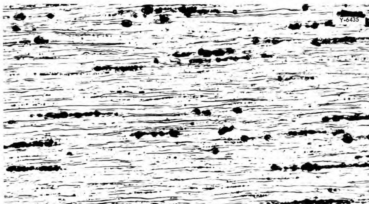
Fig. 11. Ames Thorium Cold Rolled 80%. 250X
