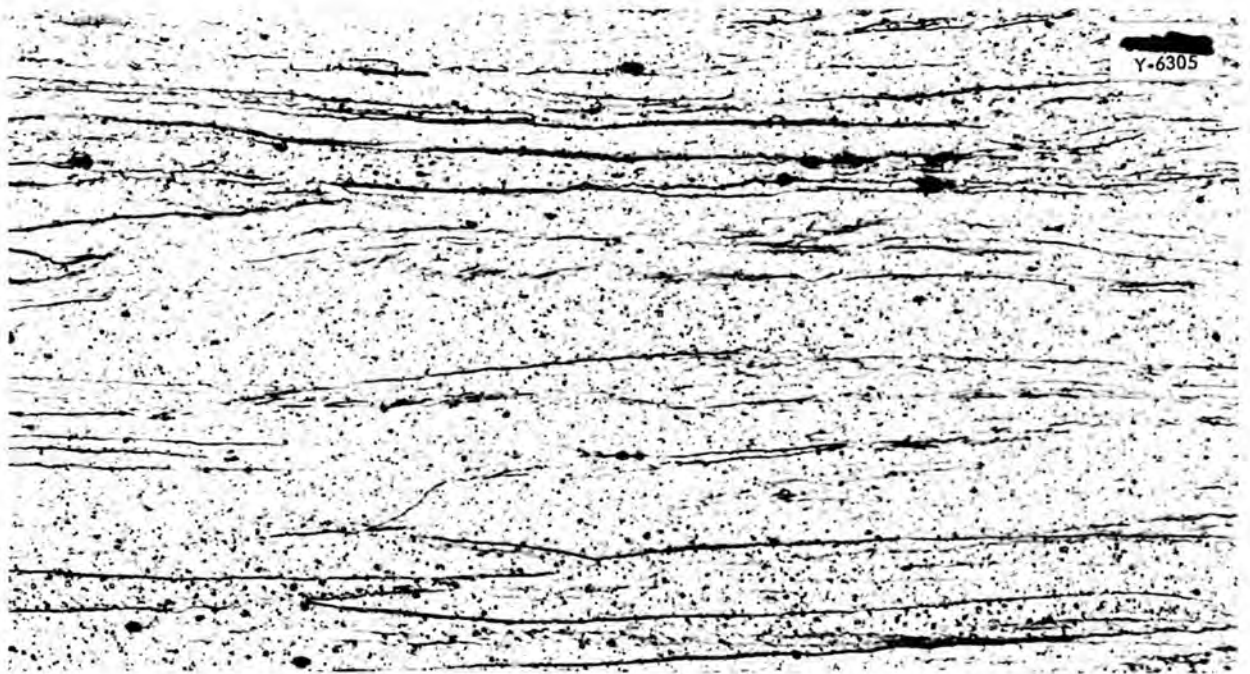
Fig. 6. Iodide Thorium Cold Rolled 80%. 250X
