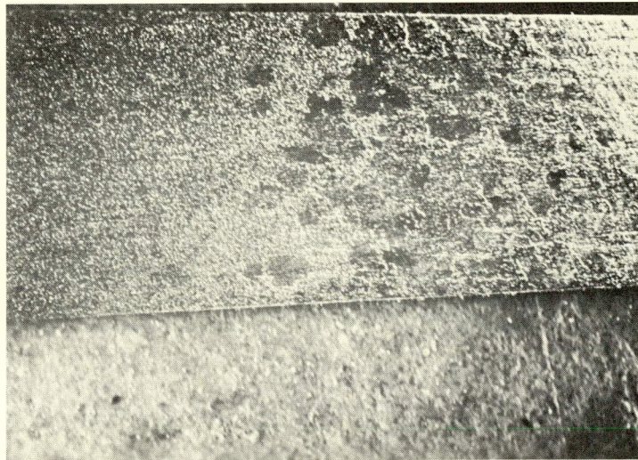
Fig. 11. The Region of Exaggerated Grain Growth in Zirconium Strained at 500^{\circ}\text{F} and Annealed for 287 Hours at 1050^{\circ}\text{F} . The critical strain for this specimen is 5 per cent elongation. 17X
