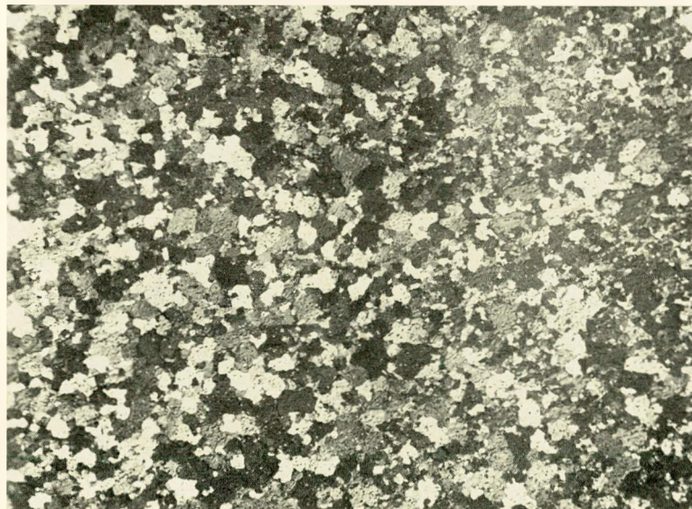
Fig. 10. Grain Growth Which Occurred at the Critical Strain in Zircaloy III Strained at 500° F and Annealed at 1050° F for 911 Hours. The critical strain is 15 per cent elongation. 50X
