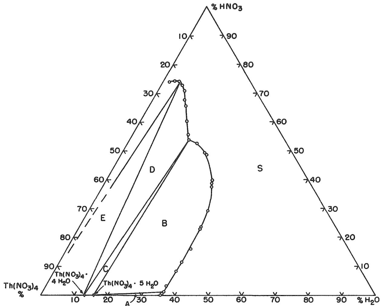
FIG. I. THE SYSTEM  $\text{Th}(\text{NO}_3)_4 - \text{H}_2\text{O} - \text{HNO}_3$  AT 25 °C.
